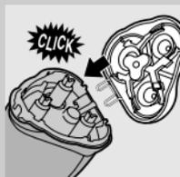
does not show any cracks or damage. If the hinge spring is still properly attached, the shaving unit can be easily put back on the shaver again. However, if the hinge spring has come loose, is cracked or damaged, please contact your Philips dealer or the nearest Philips service centre to avoid damage to your shaver.
