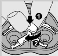
**5** Put the retaining frame back into the shaving unit, press the wheel (1) and turn it clockwise (2).
