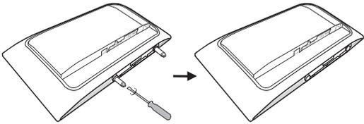
**4** Attach the supplied base cover. Your LCD TV is now ready for wall mounting.
