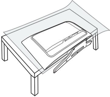
**2** Remove 3 screws from the base. Grasp the base and pull it out.
