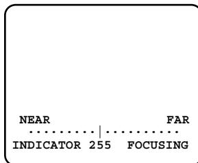
7. If needed, perform manual adjustment using the [LEFT] or [RIGHT] buttons to obtain the best focus on the targeted object while observing the picture. See the value of INDICATOR on the monitor. (The larger the value is, the better the picture quality becomes.)
