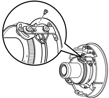
6. Secure the camera unit to the bracket with the camera lock screw.
