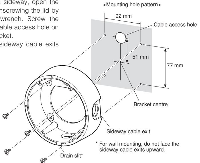
**<Fixing the camera attachment to the mounting bracket>**
