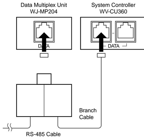
To use cables locally purchased, they must be of the data grade: BELDEN 9406 or equivalent. The pin assignments and data flow are shown below.
