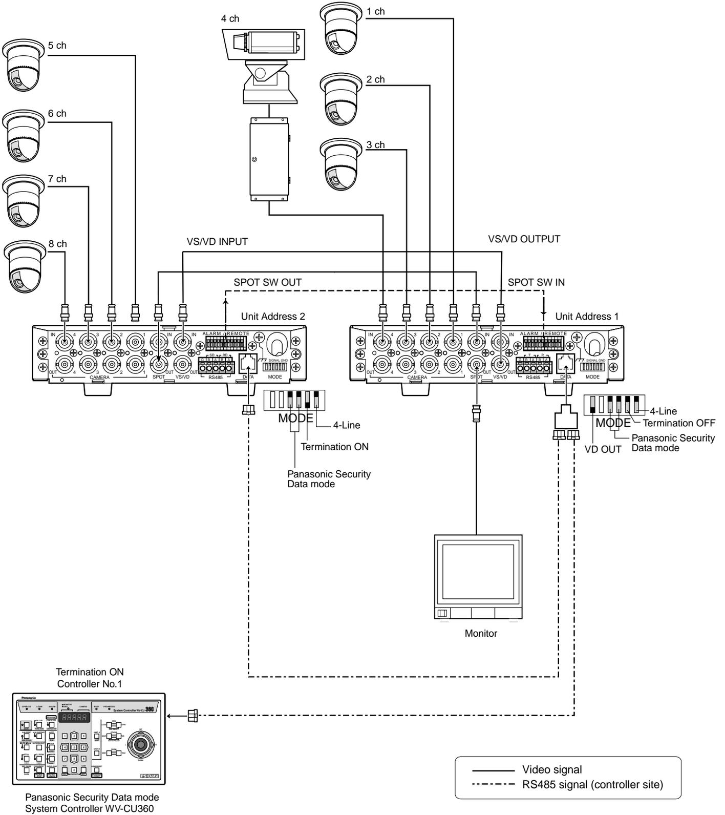
● **Connecting Two or More Data Multiplex Units to Matrix Switcher WJ-SX350 (Camera Communication Mode)**
