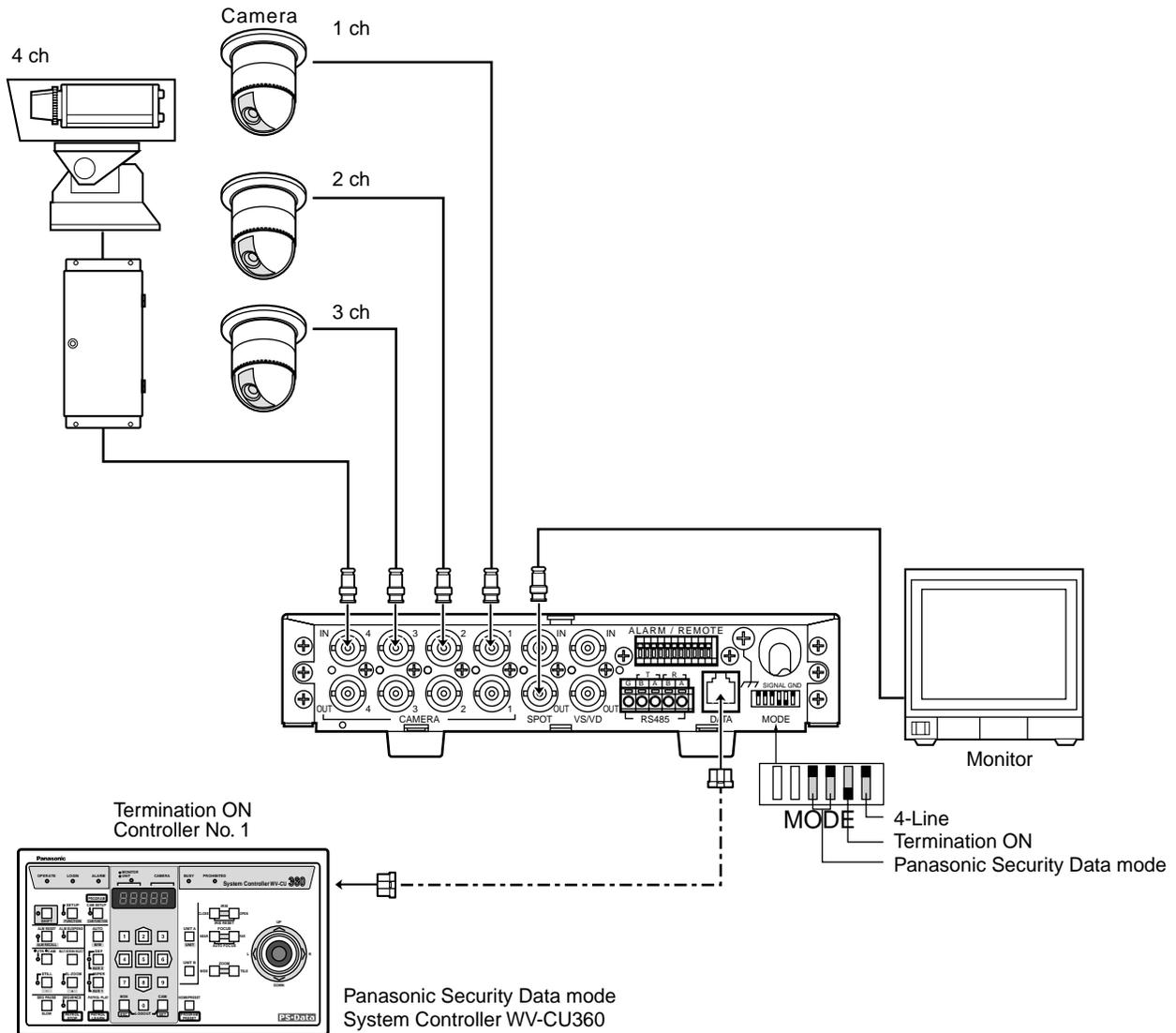
● **Connecting Two or More Data Multiplex Units to System Controller WV-CU360 (Panasonic Security Data Mode)**
