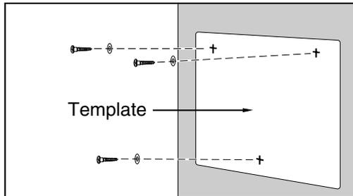
2. Drill holes in the wall as marked and fit the anchor plugs (not included) into the holes.
