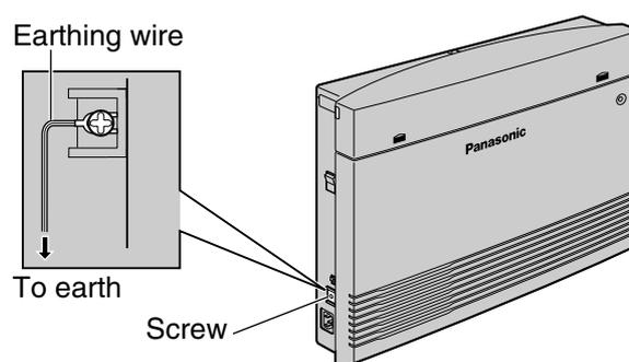
\* Use an earthing wire that has a conductor with a cross-sectional area of at least 0.75 mm<sup>2</sup> or 18 AWG. Green-and-yellow insulation is required.
