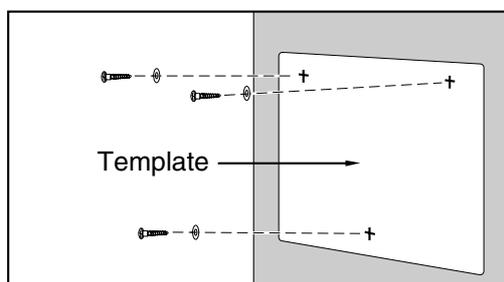
2. Fit the washers on the screws, and drive the screws into the wall.
