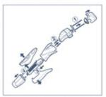
· Perform steps ① to ④ and lift the battery, and then remove it.
