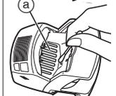
Do not pull hard on the rubber blade protector (a) at the bottom of the cleaning tray. The rubber may come off if you pull hard on it. It is only necessary to pull it up slightly.
