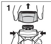
3. Align the foil frame mark (⌘) and the system outer foil mark (△) and securely attach together.
