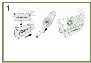
Open Micro-Pak® Sheet foil package. Remove roll of Micro-Pak® PE Sheet and place them in the Micro-Pak® dispenser box.
