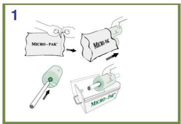
Open Micro-Pak® Sheet foil package. Remove roll of Micro-Pak® PE Sheet and place them in the Micro-Pak® dispenser box
