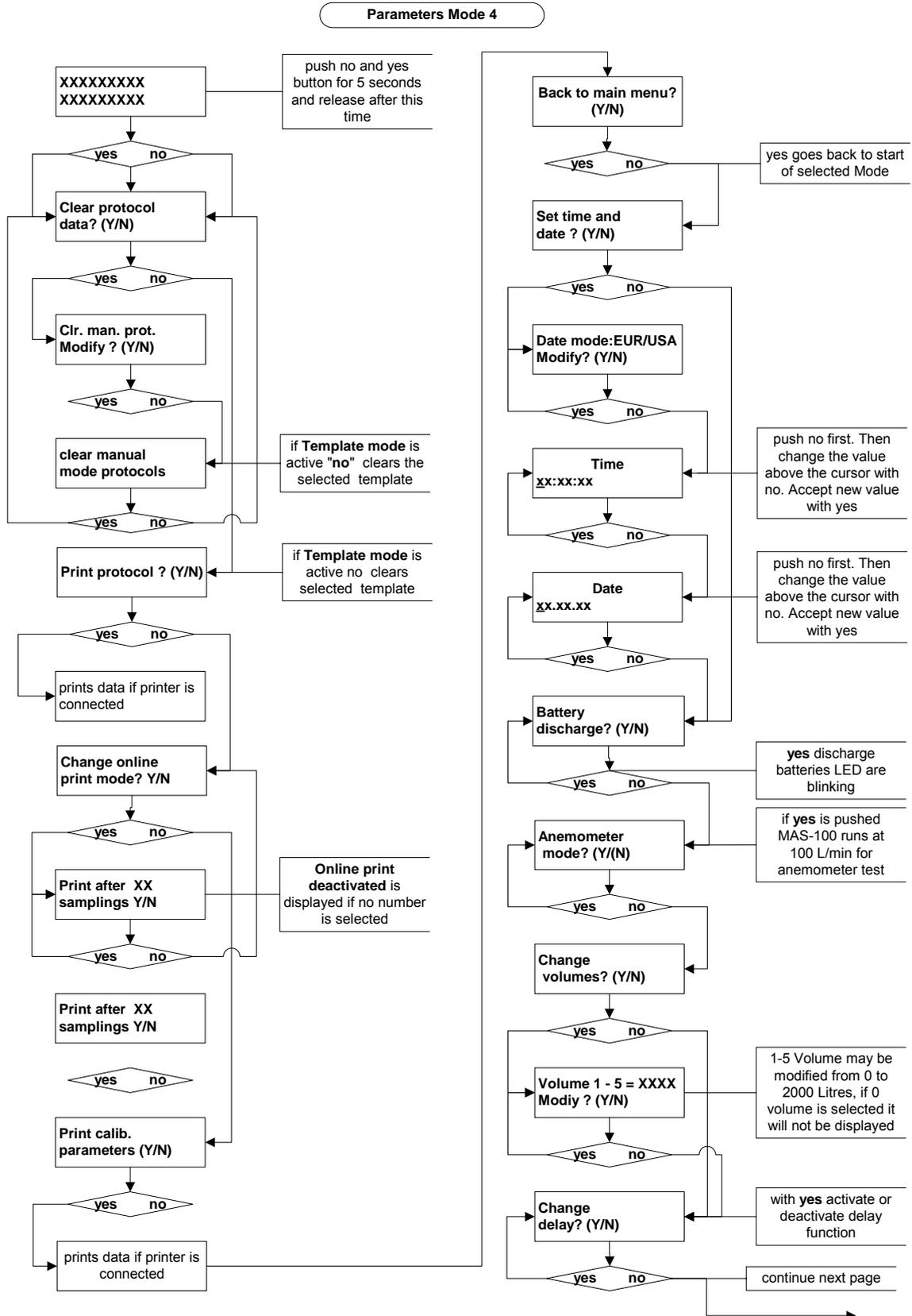
Continue: Firmware Flow Diagram MAS-100™: Parameters Mode 4
