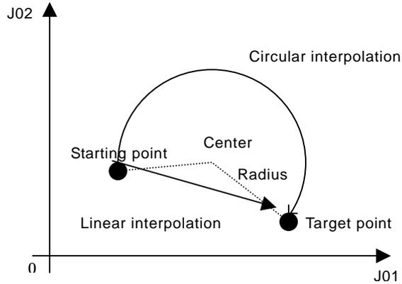
If [axis name 3] is added, helical interpolation is added to the linear interpolation. (The linear interpolation portion for multiple revolutions specifies the total travel distance.)
