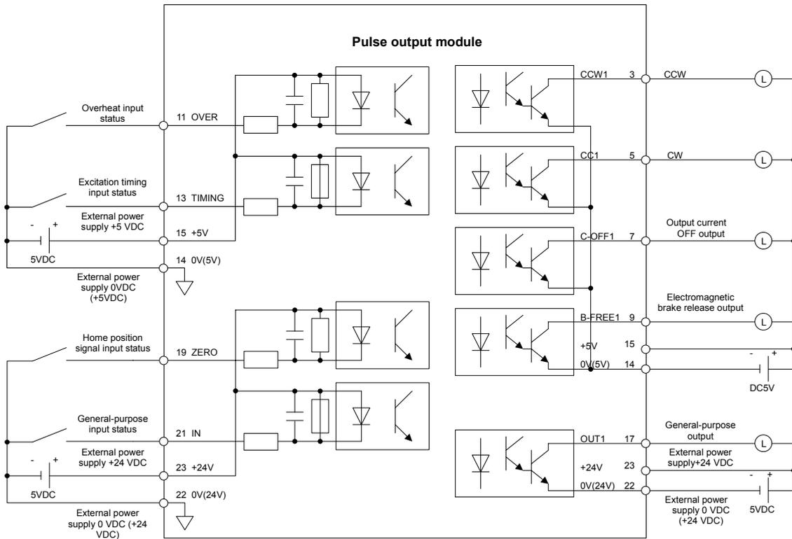
■ Signal arrangement of the terminal block
