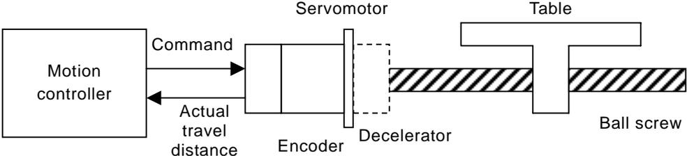
The semi-closed loop system is the mainstream in modern servo systems applied to positioning devices for industrial applications.
