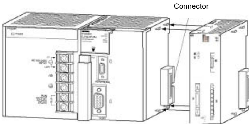
2. Secure the PCU by sliding the yellow sliders on the top and bottom unit they click into place.
