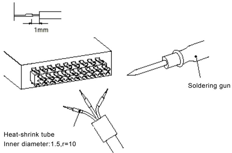
4. Pull the heat-shrink tubing back over the soldered area and heat the tubing to shrink it.
