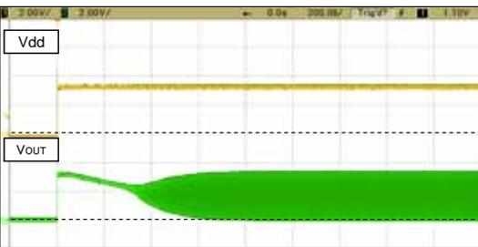
Typical sample at V<sub>dd</sub>=3.3V,25deg.C
