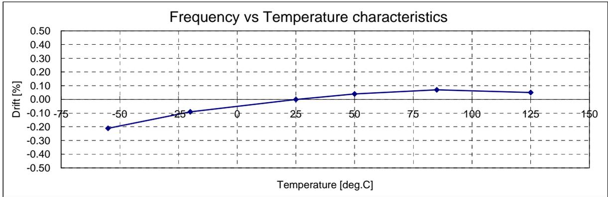
Typical sample at V<sub>dd</sub>=3.3V
