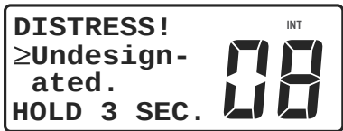
Distress Alert Screen
