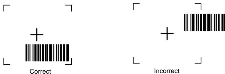
Figure 2-21 Imager Aiming Pattern: Bar Code Not Centered
