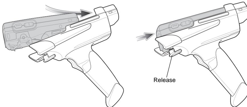
Figure 6-15 Inserting the EDA into the Trigger Handle
