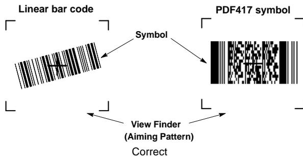
Figure 2-20 Imager Aiming Pattern: Bar Code Centered
