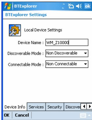
**Figure 4-34** BTE Explorer Settings - Device Info Tab
