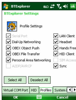
**Figure 3-4** BTE Explorer Settings - Profile Tab
