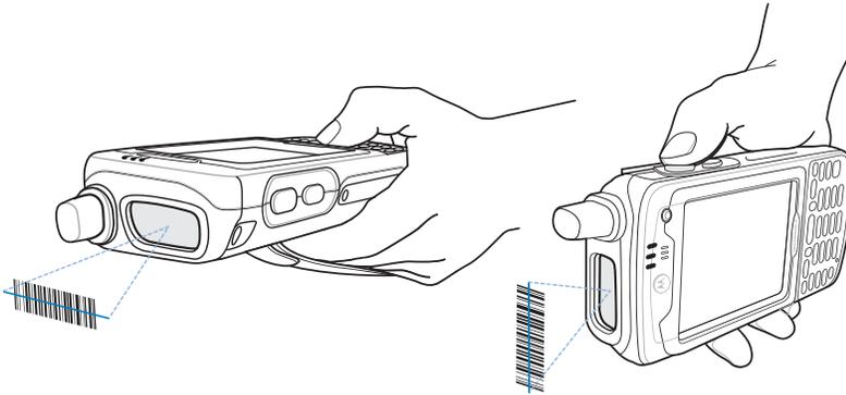
Figure 2-17 Linear Scanning
