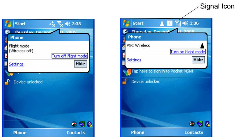
Figure 5-2 Turning Flight Mode On and Off
