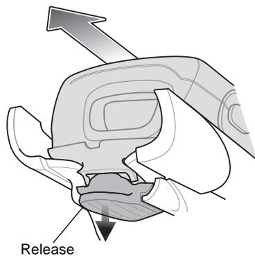
Figure 6-16 Removing the EDA
