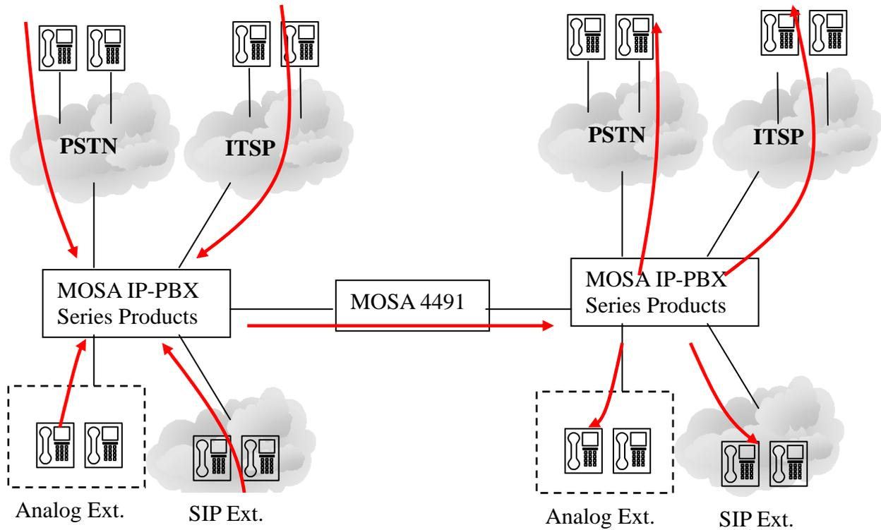
One step or 2 steps dialing incoming call from trunk (PSTN, ITSP (Internet Telephony Service Provider)) or line (Analog Ext., SIP Ext.) of MOSA IP-PBX to MOSA 4491 can be redirected to line (Analog Ext., SIP Ext.) of remote MOSA IP-PBX directly or remote trunk (PSTN, ITSP (Internet Telephony Service Provider)) of remote MOSA IP-PBX directly.
