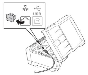
С Carefully guide the network cable into the cable channel and out the back of the machine. Connect the cable to your network.
