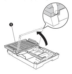
With both hands, gently press and slide the paper length guide ① and then the paper side guides ② to fit the paper size.
