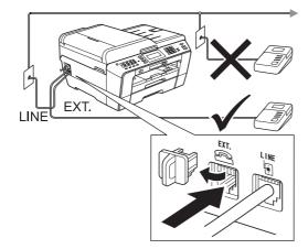
Set the receive mode to External TAD if you have an external answering machine. See Choose a Receive Mode on page 8. For additional details, see Connecting an external TAD (telephone answering device) in chapter 6 of the Basic User's Guide.
