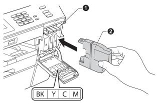
Gently push the back of the ink cartridge marked "PUSH" until it clicks. After all the ink cartridges are installed close the ink cartridge cover.
