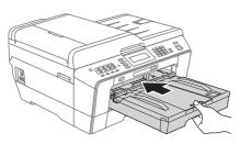
While holding the paper tray in place, pull out the paper support ① until it clicks, and then unfold the paper support flap ②.
