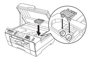
**f** Gently close the scanner cover using the finger holds on each side.
