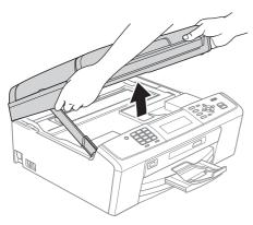
b Connect the USB cable to the USB socket marked with a symbol. You will find the USB socket inside the machine on the right as shown below.
