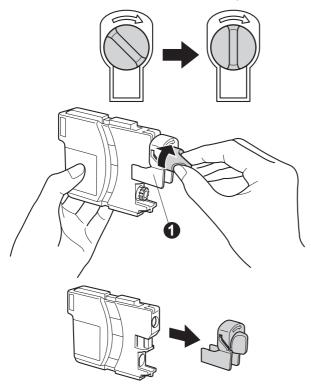
Take care to match the color of the lever with the cartridge color 2, as shown in the diagram below.
