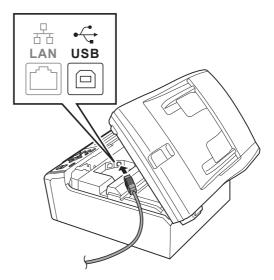
C Carefully guide the USB cable through the trench as shown below, following the trench around and toward the back of the machine. Then connect the cable to your Macintosh.
