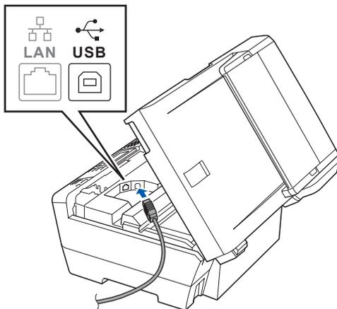
**d** Carefully guide the USB cable through the trench as shown below, following the trench around and toward the back of the machine. Then connect the cable to your computer.
