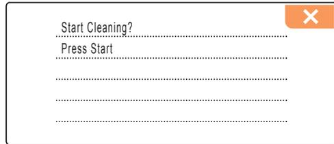
**e** Press **Color Start**, the machine will then start cleaning the colors.
