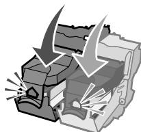
**4** Lift the scanner unit and push the scanner support back while lowering the scanner unit until it is completely closed.
