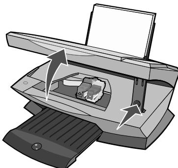
The print cartridge carrier moves and stops at the loading position unless the All-In-One is busy.
