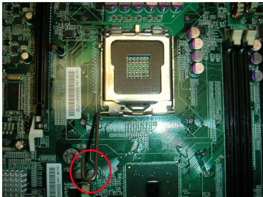
3. Now that the lever is in its unlocked position, lift up the metal cover to reveal the CPU socket.
