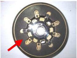
Remove the clutch pressure plate and the complete pack of disks.
