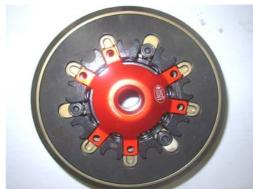
Lock the clutch with the lock wrench (provided) and remove the nut.
