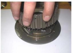
Remove the six steel balls.
