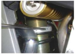
Use the supplied adjusting pin to turn the ring nut until achieving the desired spring preload.
