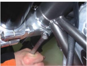
Operating on the square drive nut, turn the headstock strut by 180°.
