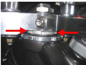
• Loosen the screw that locks the lower eccentric ring nut.
