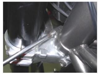
Loosen the screw that locks the upper eccentric ring nut.
