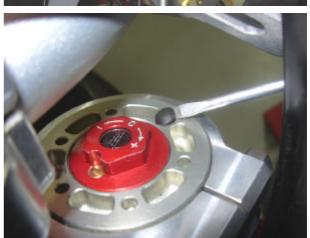
With the help of a screwdriver open the bleed valve until the air inside is completely expelled.
