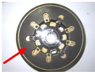
Remove the clutch pressure plate and the complete pack of disks.
