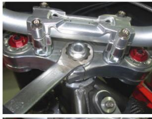
• By operating on both fork legs, loosen the tightening screws on the upper plate.
