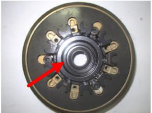
Remove the thrust ring.
