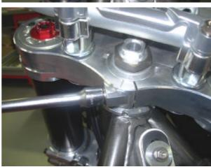
Loosen the screw that closes the lower plate.
