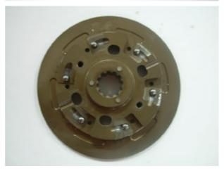
The two springs can be replaced with springs with a different elastic constant K to adapt the response of the clutch to its requirements.
