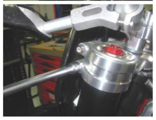
Slightly lift the upper plate, by pulling it out by a few millimetres from the fork legs.
