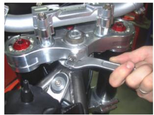
The ring nut to work on is the upper one, immediately below the steering plate.
