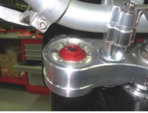
Using a hook spanner, loosen the bearings preload ring nut
