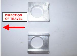
• Mount the chain tensioner pads in the direction indicated when installing the sprocket with less teeth.
