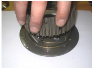
Remove the six steel balls.
