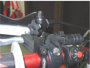
Use the adjustment knob on the left handlebar until the desired distance is obtained.
