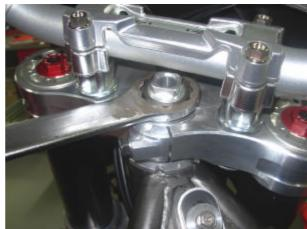
Loosen the screw that closes the upper plate.
