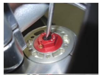
In order to adjust the hydraulic brake in extension operate on the screw shown to the side.
