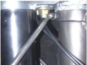
Using a hook spanner, turn the upper eccentric ring nut by 180°.
