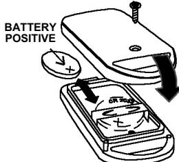
You should replace the battery with a new CR 2032 3V Lithium battery (item code 222120050).
