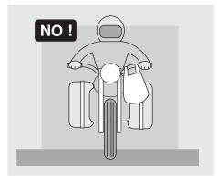
Avoid hanging bulky, heavy and/or dangerous objects on the handlebars, mudguards and forks, because the vehicle might respond more slowly in turns and its manoeuvrability could be unavoidably impaired.
