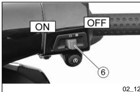
The engine stop switch «6» is to be used in emergency or dangerous situations. With the switch «6» set to «ON» is possible to start the engine; by turning it to the «OFF» position, the engine stops.
