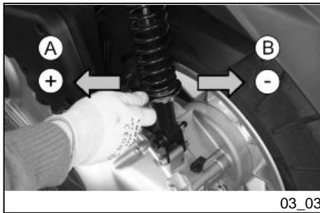
Turning the ring nut towards **A**: increases spring preloading. The scooter suspension is very hard. To be used on even or ordinary surfaces or when riding with passenger.
