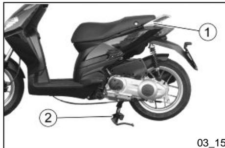
**Stand (03\_15, 03\_16)****PLACING THE VEHICLE ON THE CENTER STAND**
