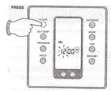
Step 2: Press the CLOCK button again and "12:" (hours) and "AM" or "PM" will flash. Use the DECREASE or INCREASE button to change the flashing symbol to the current hour making sure the hour has the proper AM or PM designation.
