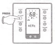
Step 2: To set all program temperatures, press and release the SET TEMP button. The Morning "\_\_\_\_\_" event symbol and flashing temperature will appear on the display.
