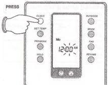
**Step 4:** Press the **CLOCK** button again. The clock is now set and the current time appears on the display.
