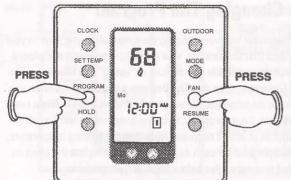
To activate the progressive recovery mode simultaneously press the **PROGRAM** and **FAN** buttons. A small thermostat icon, " ", will appear under the clock. Once in this mode proceed with programming your thermostat remembering to use exact times for each event time change.
