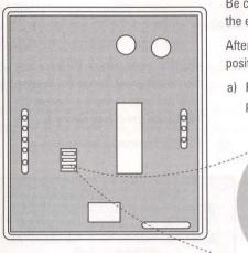
Be careful to change only the intended DIP switches per the explanation given at the beginning of this section.
