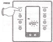
**Step 5:** Press the **CLOCK** button again. The clock is now set and the current time appears on the display.
