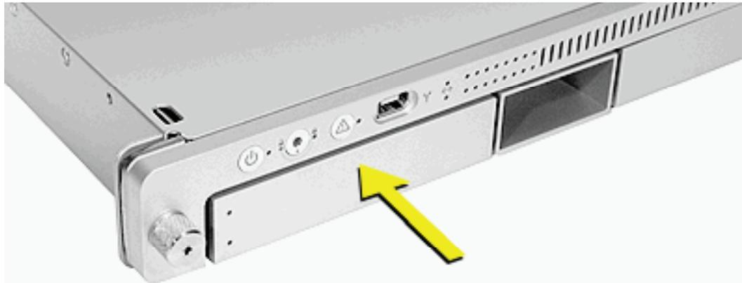
3. Wait for the upper LED on the drive to go out. Then grasp the drive handle, and pull the drive module out of the server.
