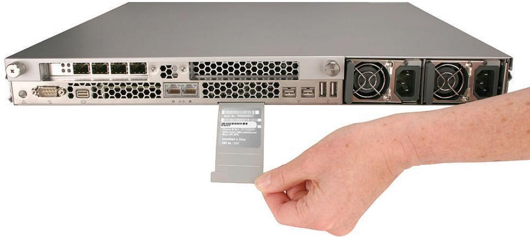
1. Locate the rear ID tab. Once the logic board has been removed from the enclosure, the ID tab is visible on the inside bottom of the enclosure.
