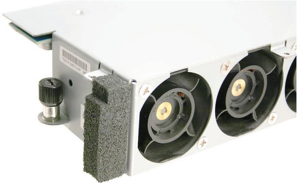
2. Align the power connector on the fan array with its connector on the power distribution board and lower the array into the enclosure. Push down on the fan array power connector to make sure it is fully seated.
