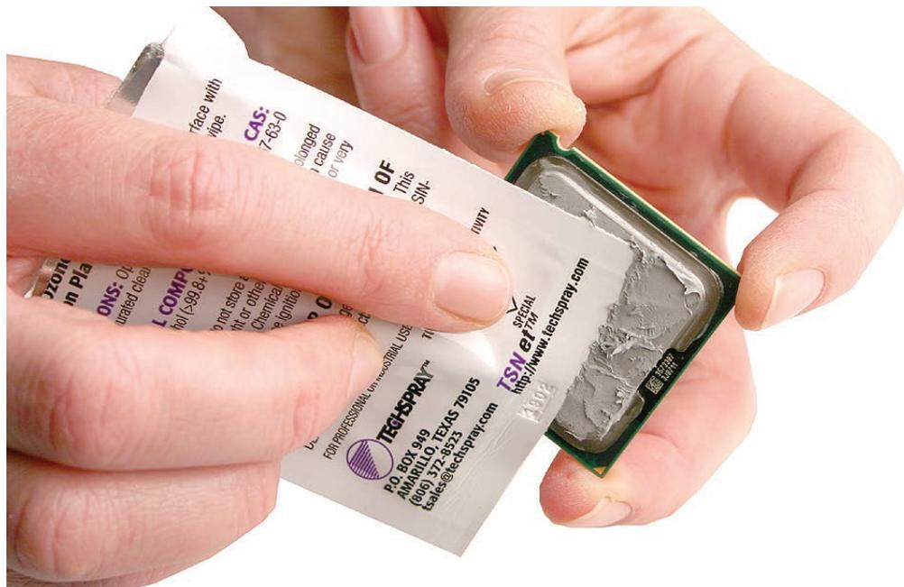
7. Holding the processor by three corners only, keep the processor level as you place it into its holder on the logic board, being careful not to get any thermal grease on the contacts of either the processor or its socket holder.
