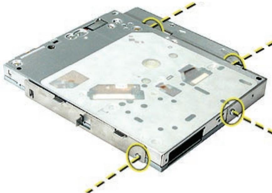
3. Slide the replacement drive into the server, making sure the tabs on the bottom edges of the drive brackets engage with the slots in the drive bay.
