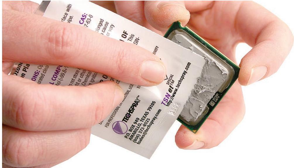
7. Holding the processor by three corners only, keep the processor level as you place it into its holder on the logic board, being careful not to get any thermal grease on the contacts of either the processor or its socket holder.
