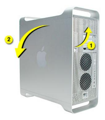
3. Install the replacement access panel by inserting the tab on the bottom edge of the panel into the channel in the bottom frame of the enclosure. Then rotate the panel up flush against the top frame.
