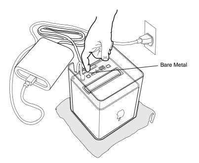
**Important:** To avoid electrostatic discharge, always ground yourself by touching the port access covers before you touch any parts or install any components inside the computer. To avoid static electricity building back up in your body, do not walk around the room until you have completed the installation and closed the computer.
