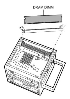
Your computer uses synchronous DRAM (SDRAM) DIMMs that must be compatible with the computer's specifications. Replace the DIMM in your computer with the replacement DIMM provided in this package. Do not use DRAM DIMMs from older computers, even if they fit into the DIMM slots.
