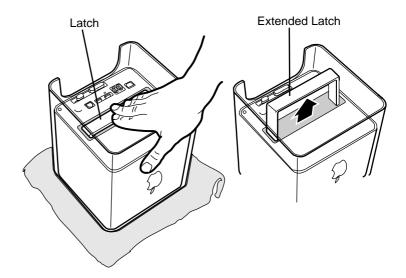
Allow the latch to extend completely.
