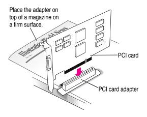
8 Align the PCI card and the adapter over the PCI slot.
