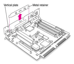
5 Remove the PCI card adapter from the main logic board.
