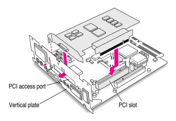
Insert the adapter into the PCI slot on the main logic board. Make sure the metal fence on the PCI card engages the hook on the vertical plate and that any connectors on the card protrude through the PCI access port opening.
