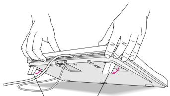
To adjust the keyboard angle, lower the feet until they snap into position.
