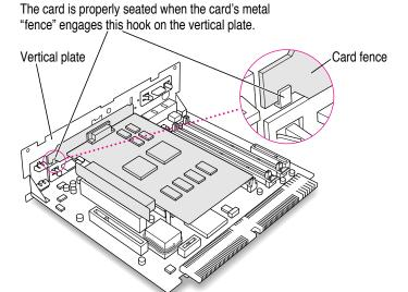
If you meet resistance, pull the adapter out and try again. To see if the adapter is properly connected, lift it gently. If it resists and stays in place, it's connected.
