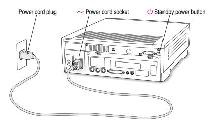
WARNING This equipment is intended to be electrically grounded. Your Macintosh is equipped with a three-wire grounding plug—a plug that has a third (grounding) pin. This plug will fit only a grounded AC outlet. This is a safety feature. If you are unable to insert the plug into the outlet, contact a licensed electrician to replace the outlet with a properly grounded outlet. Do not defeat the purpose of the grounding plug!
