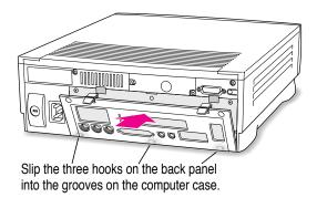
5 Swing the back panel up and snap it into place.
