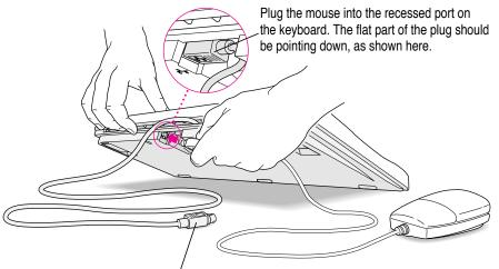
This cable plugs into the Apple Desktop Bus (ADB) port, marked with the  $\Im$  icon, on the back of the computer.
