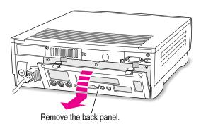
If there are security screws on the vertical plate on the back of the computer, remove them with a screwdriver.
