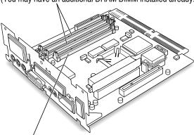
Cache slot for installing a High Performance Module for additional processing power
