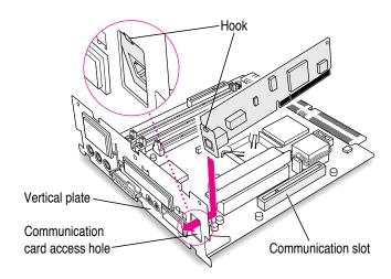
If the card does not have a hook, simply pass the external connector through the opening in the vertical plate as shown. (Some cards have a flat external connector.)
