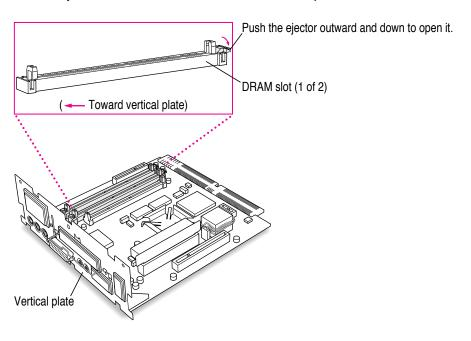
With the ejector in the "open" position, align the DRAM DIMM in one of the slots as pictured.
