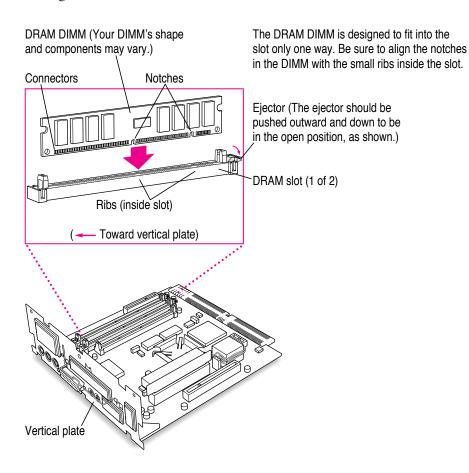
3 Push down on the DIMM until it snaps into place.
