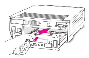
9 Once the logic board is out, set it on a clean, flat, stable surface. Rest the end of it on a thick magazine or a thin book to protect the components underneath.
