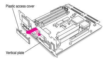
4 Remove the metal retainer from the inside of the vertical plate.
