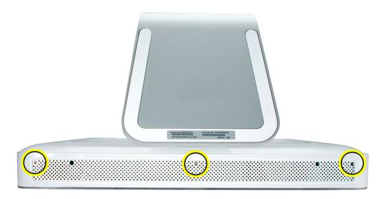
6. Holding the stand, tilt the back cover up and lift it off the computer.
