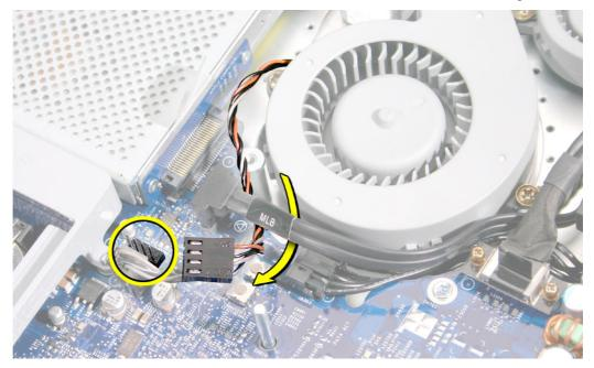
5. Route the fan cable under the black cable. Connect the fan cable to the logic board.
