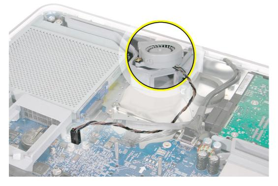
11. Remove the screws from the fan grommets. Using a screwdriver, push the fan screws out of the grommets and set them aside.
