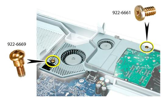
4. Using the tool provided (Torx or Phillips), loosen the two fan screws. **Note:** You don't have to remove the screws from the rubber grommets to remove the fan, just loosen the screws.
