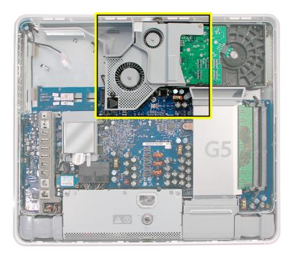
3. Using the tool provided, or a Phillips #2 screwdriver, remove the two fan cover screws. Lift the fan cover off the computer and set the fan cover aside.
