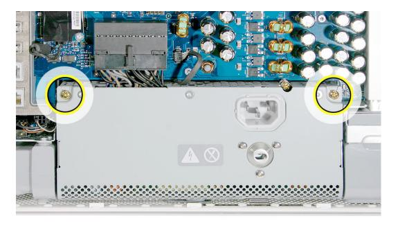
4. Loosen the middle power supply screw (also a captive screw) by turning it to the left until it is flush with the top of the power supply. This screw attaches the power supply to the display bezel below; make sure to loosen the screw all the way.
