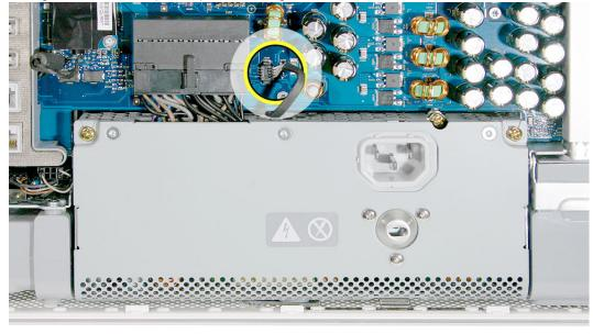
6. Turn the middle case screw clockwise about five revolutions. This releases the back cover clamp screw.
