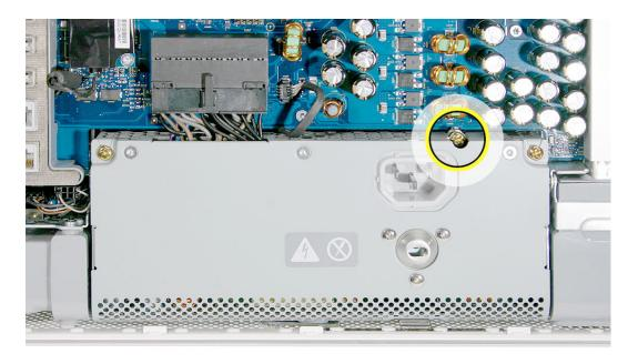
10. Turn the middle case screw to the left about five revolutions. This step prepares the back cover for installation.
