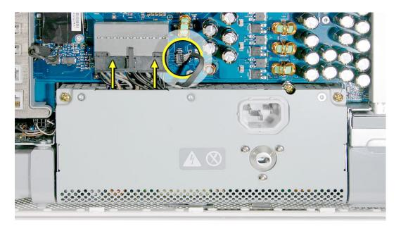
8. Tighten the two outer captive screws, turning them to the right
