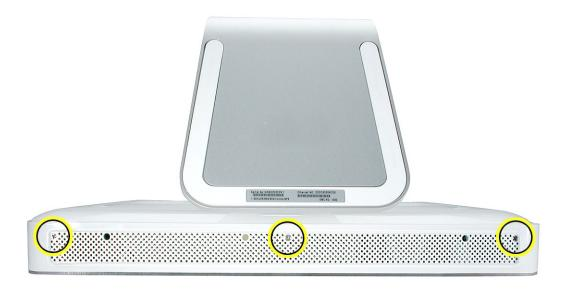
4. Position the computer in the upright position. Reconnect the power cord and remaining cables. Turn on the computer.
