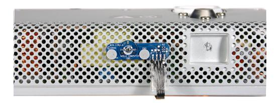
3. Push the center screw up with a flat-blade screwdriver. It will be easier to install the power supply with the screw pushed up and out of the way.
