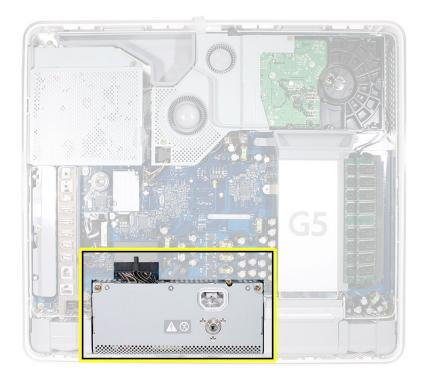
3. Loosen the two outer power supply screws by turning them to the left. **Note:** These screws are captive; they cannot be removed.
