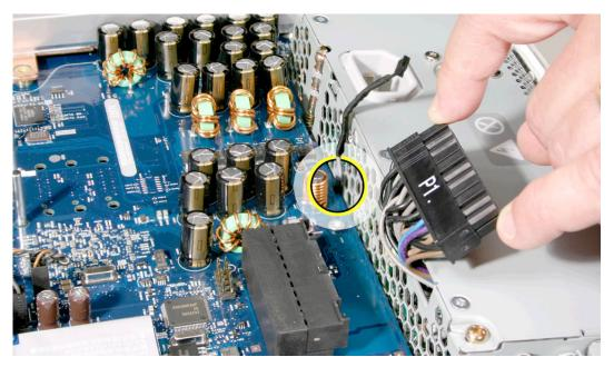
7. Connect the black power supply cable and the ambient light sensor (if you have one).
