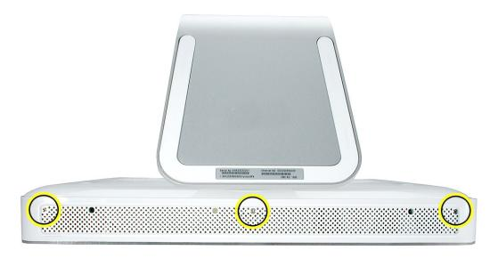
5. Holding the foot, tilt the back cover up and lift it off the computer.
