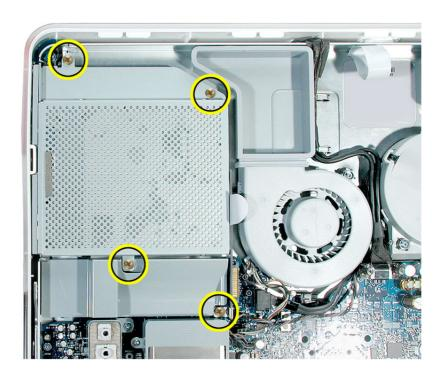
4. Pull the optical drive tab straight up and then to the right. Set the optical drive aside.
