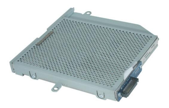
10. With your thumb on the pull tab and your index finger behind the tab, push the optical drive in the direction of the arrow and then push down to seat the drive.
