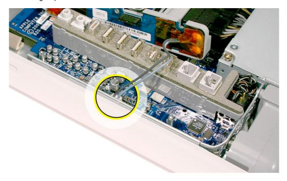
11. Turn over the inverter as shown. Using your fingers or a flat-blade screwdriver, remove the gray plastic inverter cover by gently prying the tabs (circled below) away from the board. **Note:** Return the inverter board to Apple in the packaging provided.
