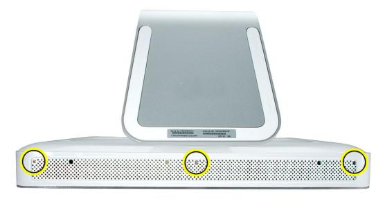
5. Holding the back cover by the metal stand, tilt the cover up and lift it off the computer. Set the back cover aside.
