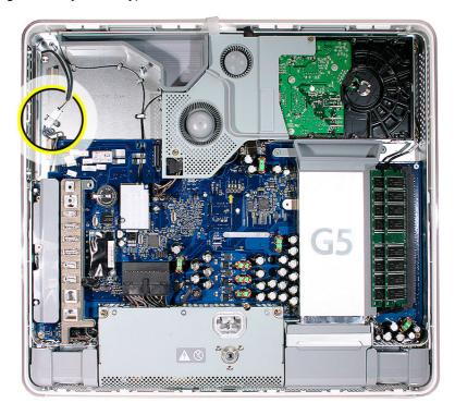
8. Tuck the white connector under the metal tab and route the cable (near the top of the inverter board) under the logic board.
