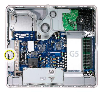
7. Reconnect the inverter-to-display panel cable. **Important:** The connector is keyed (it fits together only one way).
