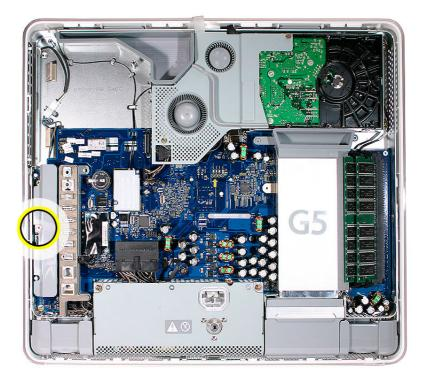
9. Lift the inverter straight up to disconnect the inverter board.
