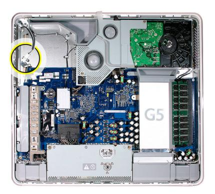
7. Release the cable from the clip. Disconnect the cable connector.
