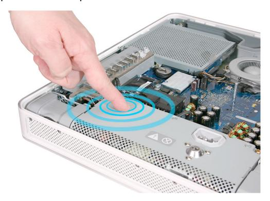
3. Locate the AirPort Extreme card. The battery is located below the AirPort Extreme card. **Note:** If an AirPort Extreme card is not installed, go on to step 7.
