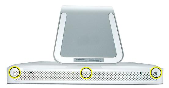
5. Holding the back cover by the metal stand, tilt the cover up and lift it off the computer. **Important:** Return this back cover and stand to Apple in the packaging provided.
