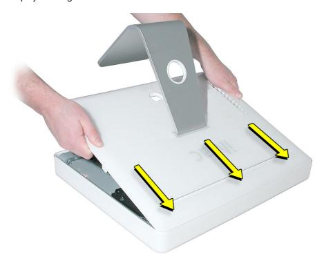
2. Lower and press the cover into place until it fits snugly on the computer.
