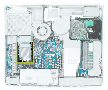
3. Disconnect the antenna cable from the end of the installed AirPort Extreme card.
