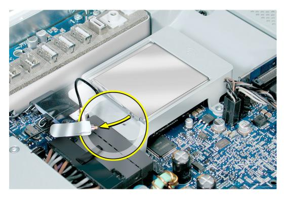
Pull the tab on the card to remove the card from the AirPort card guide.
