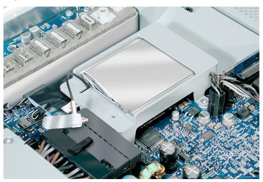
3. Connect the antenna cable to the end of the installed AirPort Extreme card.
