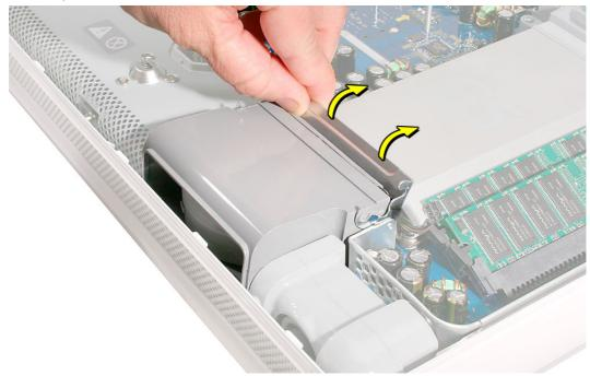
4. Disconnect the fan connector on the logic board. Pull on the black connector not the cable.
