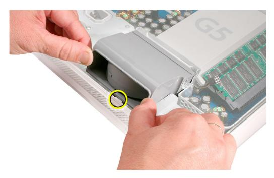
7. Pull the fan cable through the metal bracket (1) as you pull the fan forward (2).
