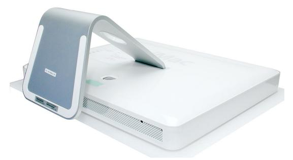
4. Locate the three silver case screws circled below. Lift the stand up to locate the middle case screw. **Note:** These screws are captive; they are part of the display/bezel assembly and cannot be removed.
