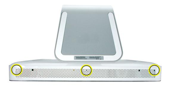
5. Holding the stand, tilt the back cover up and lift it off the computer.
