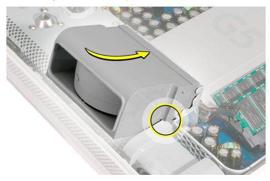
As you push the fan, make sure it clears the white tab on the display bezel.
