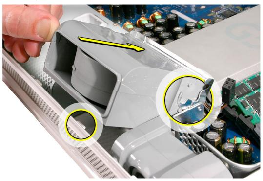
4. Lower the fan into the display bezel. Pull the metal locking clip down onto the fan making sure it secures the fan.
