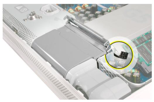
5. Grab the fan by the sides and wiggle the fan upward. As the fan comes up, the fan will bump into a tab on the front bezel. See the next step.
