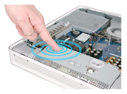
2. Locate the metal locking clip on the top of the fan housing. Use a flat-blade screwdriver to raise up the clip approximately 1/4 inch.
