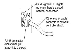
Turn on the computer's power switch, start up the computer, and check that the card's green light-emitting diode (LED) is on.
