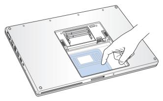
3 If you need to remove a memory card that's already installed in the slot, spread the tabs in the slot away from the notches in the memory card. The card should pop up slightly. Lift the memory card to a 25-degree angle and then gently slide the card out of the memory slot.
