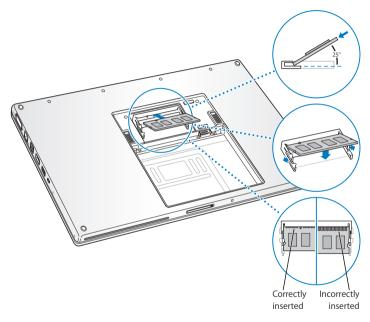
*Note:* Make sure your memory is installed according to this illustration, so the gold contacts are almost completely inserted into the connector.
