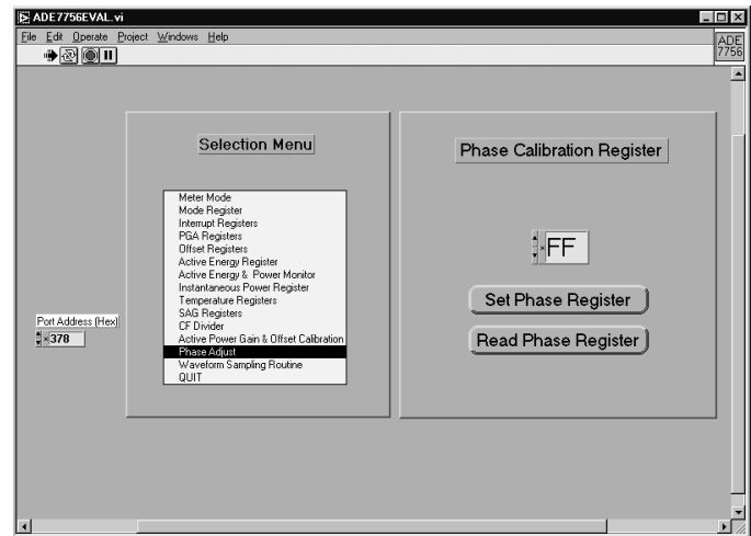
Figure 11—Writing to the PHCAL register to correct phase error
