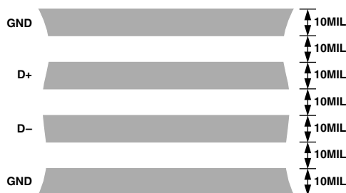
Figure 4. Arrangement of Signal Tracks
