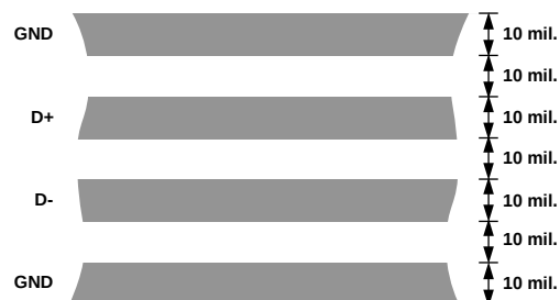
Figure 17. Arrangement of Signal Tracks
