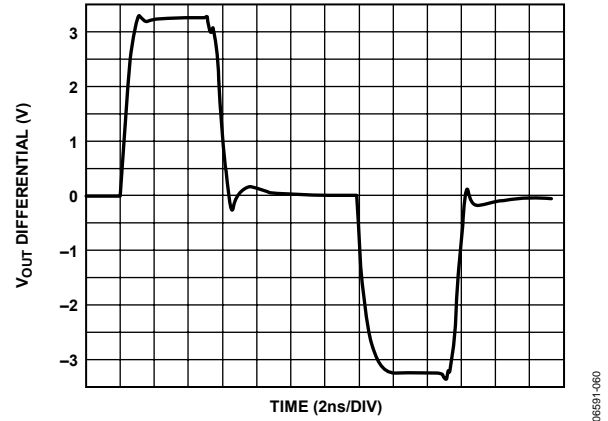
Figure 33. Overdrive Recovery Time (Pulse Input)
