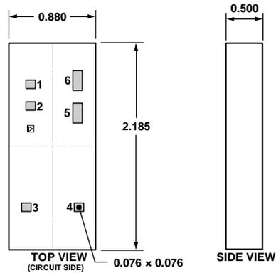
Figure 5. 6-Pad Bare Die [CHIP]
