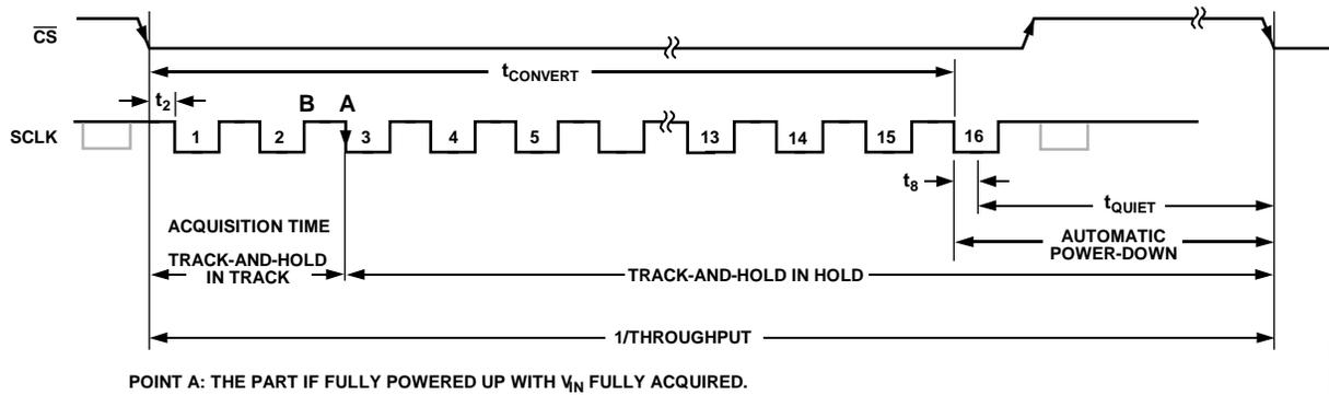
Figure 3. AD7466-KGD Serial Interface Timing Diagram Example
