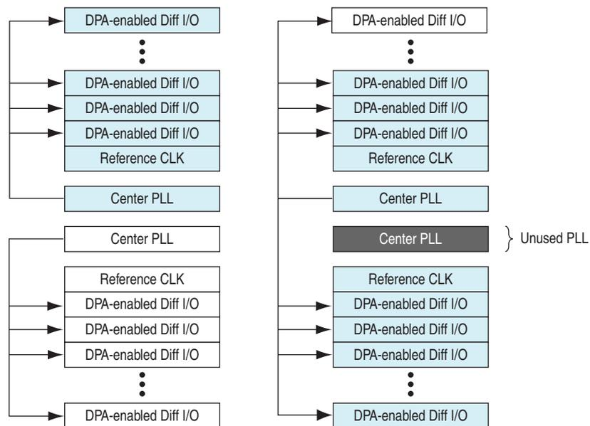
If the upper center PLL drives the DPA-enabled channels in the lower I/O bank, the lower center PLL cannot drive the DPA-enabled channels in the upper I/O bank, and vice versa. The center PLLs cannot drive cross-banks simultaneously, as shown in Figure 6-23.
