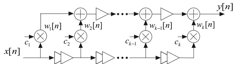
Arria V variable-precision DSP blocks support 18-bit and 27-bit systolic FIR structures.
