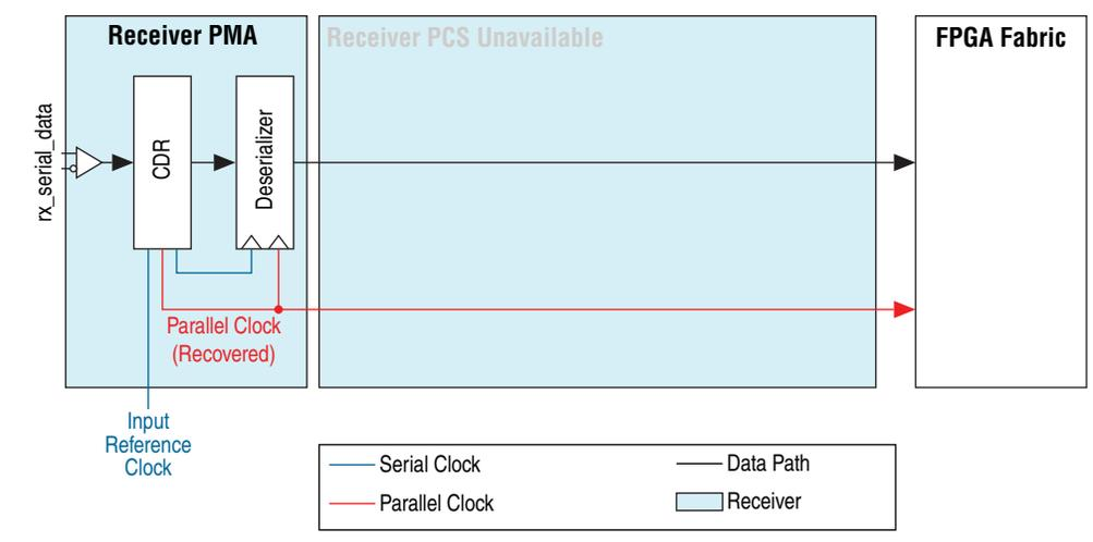
As shown in Figure 2-16, the parallel recovered clock from the CDR and deserializer is directly connected to the FPGA fabric because the PCS is unavailable in 10-Gbps transceivers. All PCS functions, such as word alignment, rate matching, decoding, and byte ordering, must be implemented in the core IP.
