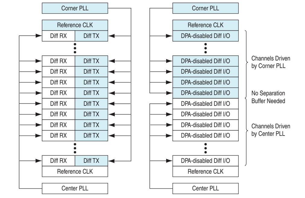
A corner PLL and a center PLL can drive duplex channels in the same I/O bank if the channels that are driven by each PLL are not interleaved. You do not require separation between the group of channels that are driven by the corner and center, left and right PLLs. Refer to [Figure 6-25](#) and [Figure 6-26](#).
