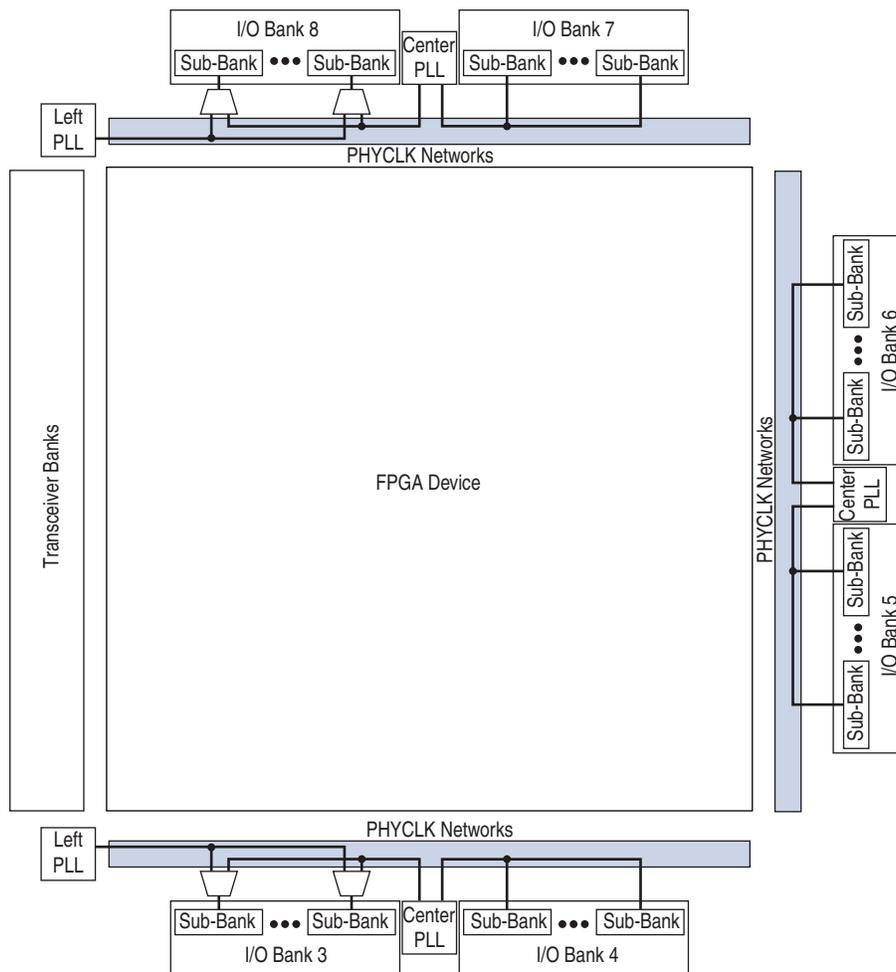
Figure 7-7. PHYCLK Networks in Arria V GX B1, B3, A5, A7, B5, and B7 Devices
