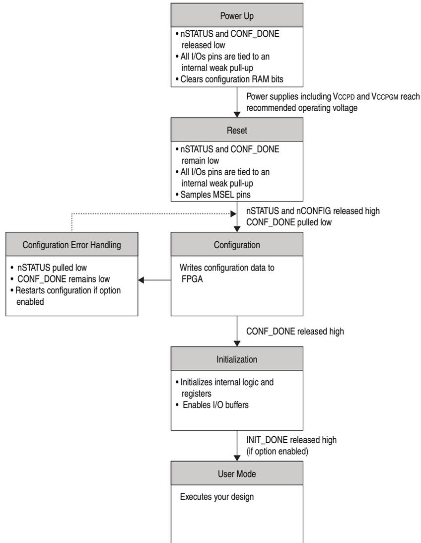
You can initiate reconfiguration at any stage by pulling the nCONFIG pin low to at least the minimum  $t_{CFG}$  low-pulse width. When this pin is pulled low, the nSTATUS and CONF\_DONE pins are pulled low and all I/O pins are tied to an internal weak pull-up.
