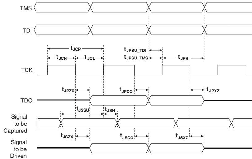
To start an IEEE Std. 1149.1 operation, select an instruction mode by advancing the TAP controller to the shift instruction register (SHIFT\_IR) state and shift in the appropriate instruction code on the TDI pin.
