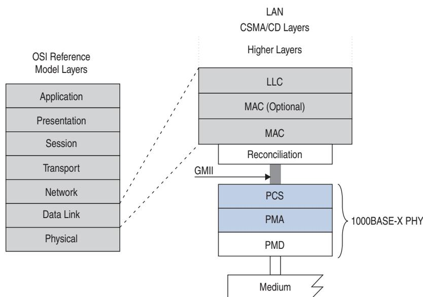
Arria V transceivers, when configured in GbE functional mode, have built-in circuitry to support the following PCS and PMA functions, as defined in the IEEE 802.3 specification:
