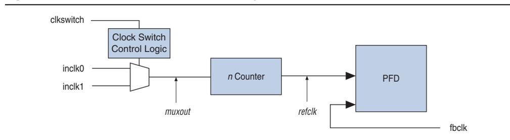
You can delay the clock switchover action by specifying the switchover delay in the `ALTERA_PLL` megafunction. When you specify the switchover delay, the `clkswitch` signal must be held high for at least three `inclk` cycles plus the number of the delay cycles that has been specified to initiate a clock switchover.
