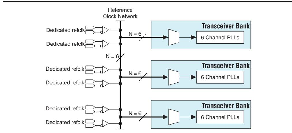
Arria V GT devices use the same dedicated `refclk` input pins as the 6-Gbps transceiver channels. For 10-Gbps channel operation, each dedicated `refclk` input pin drives only the 10-Gbps channels PLLs located in the same triplet.
