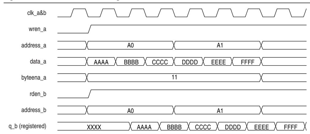
Figure 2-5 shows a sample functional waveform of mixed-port read-during-write behavior for the “old data” mode.
