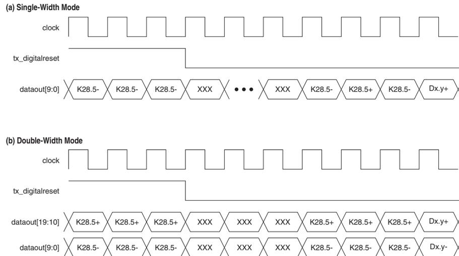
Table 1–10 lists the 8B/10B encoder output during and after reset conditions.
