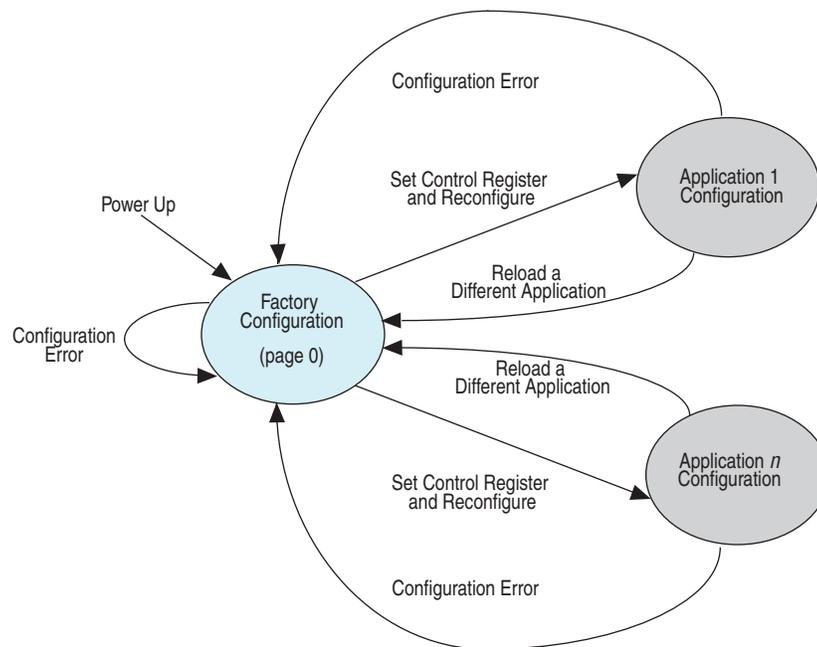
Refer to “Remote System Upgrade State Machine” on page 8-36 for a detailed description of this sequence.
