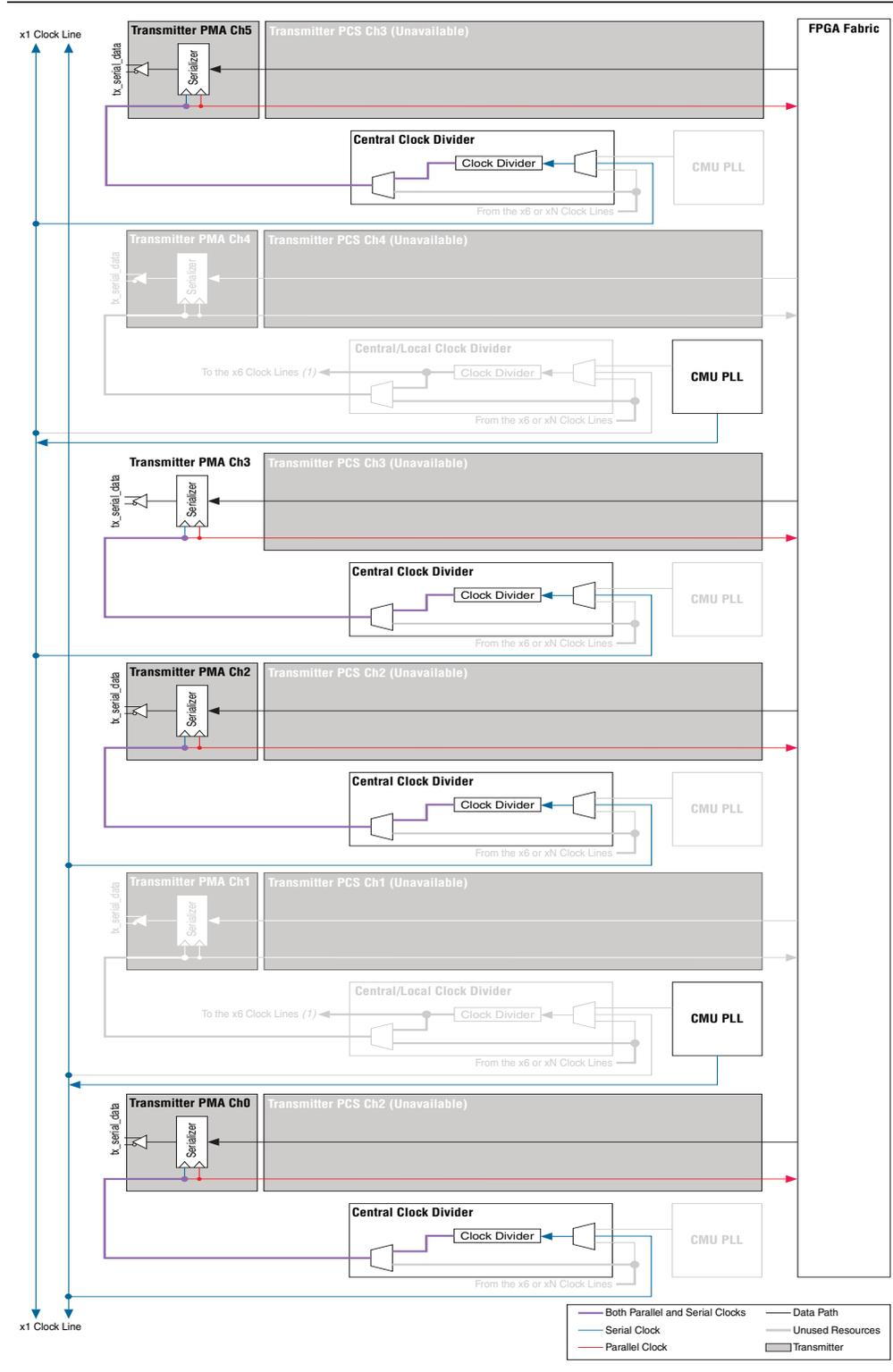
As shown in [Figure 2-12](#), the clock divider block provides the serial and parallel clock to the serializer of the transmitter PMA. The parallel clock is driven directly to the FPGA fabric because the PCS is unavailable in 10-Gbps transceivers. All PCS functions, such as encoding and bit slipping, must be implemented in the core IP.
