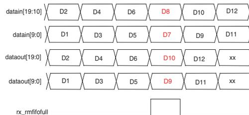
Figure 5-13 shows the rate match FIFO empty condition in custom double-width mode. The rate match FIFO becomes empty after reading out the 20-bit word D5D6.
