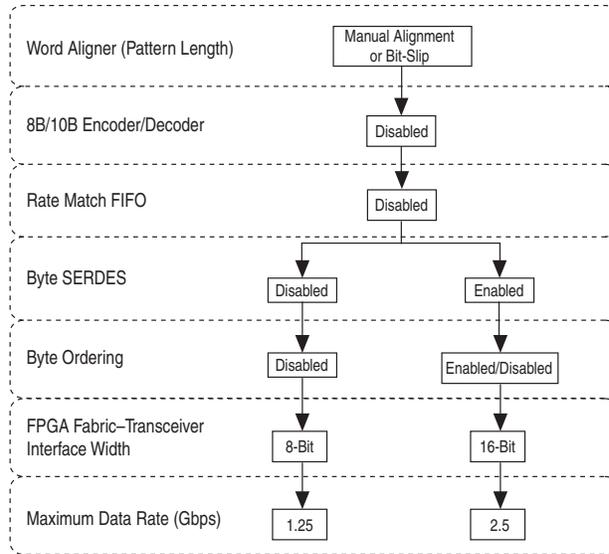
**Figure 5-3. Configuration Options for Custom Single-Width Mode (10-bit PMA-PCS Interface Width)**
