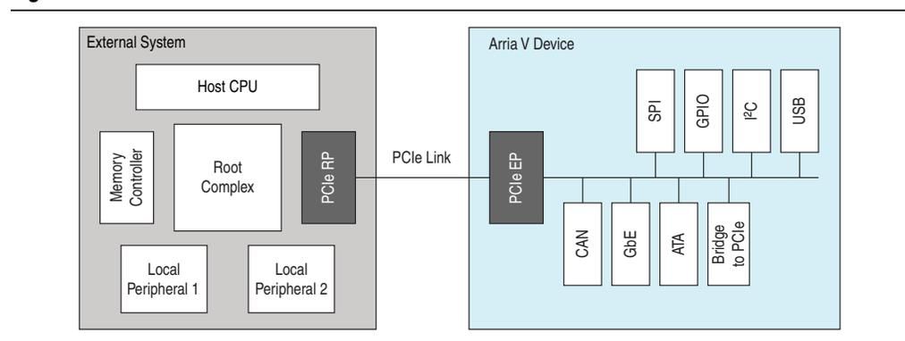
The Arria V PCIe hard IP operates independently from the core logic, which allows the PCIe link to wake up and complete link training in less than 100 ms while the Arria V device completes loading the programming file for the rest of the device.
