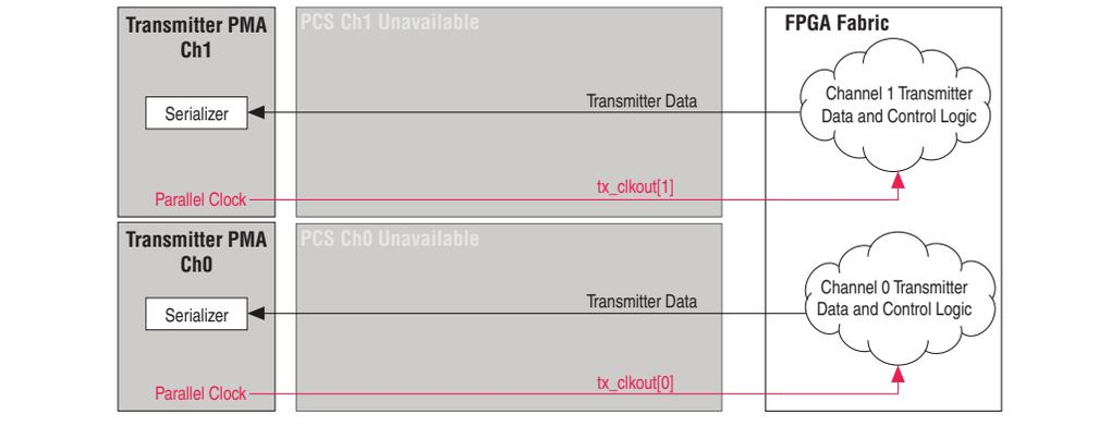
Figure 2-24 shows the 6-Gbps transmitter datapath interface of three bonded channels clocked by the `tx_clkout[0]` clock. The `tx_clkout[0]` clock is derived from the central clock divider of channel 1 or 4 in a transceiver bank.
