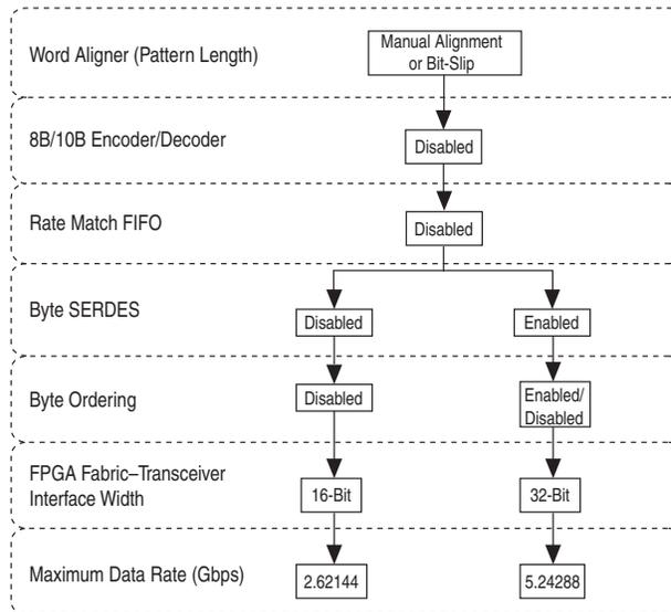
**Figure 5-5. Configuration Options for Custom Double-Width Mode (20-bit PMA-PCS Interface Width)**
