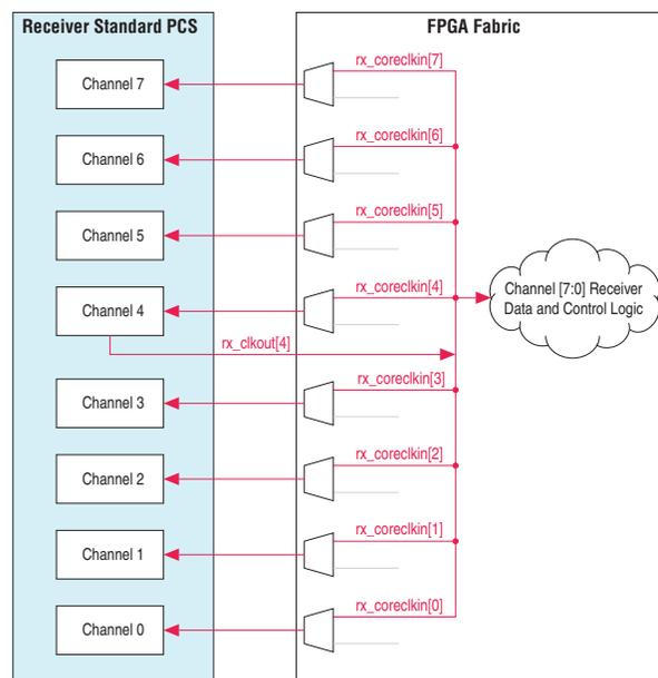
To clock eight identical channels with a single clock, perform these steps:
