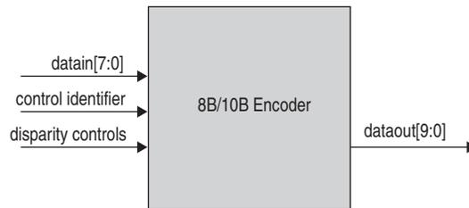
The IEEE 802.3 specification identifies only 12 sets of 8-bit characters as /Kx.y/. If other sets of 8-bit characters are set to encode as special control code-groups, the 8B/10B encoder may encode the output 10-bit code as an invalid code (it does not map to a valid /Dx.y/ or /Kx.y/ code), or unintended valid /Dx.y/ code, depending on the value entered.
