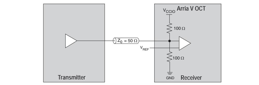
R<sub>T</sub> OCT with calibration is available only for configuration of input and bidirectional pins. Output pin configurations do not support R<sub>T</sub> OCT with calibration. When you use R<sub>T</sub> OCT, the  $V_{CCIO}$  of the bank must match the I/O standard of the pin where you enable the R<sub>T</sub> OCT.
