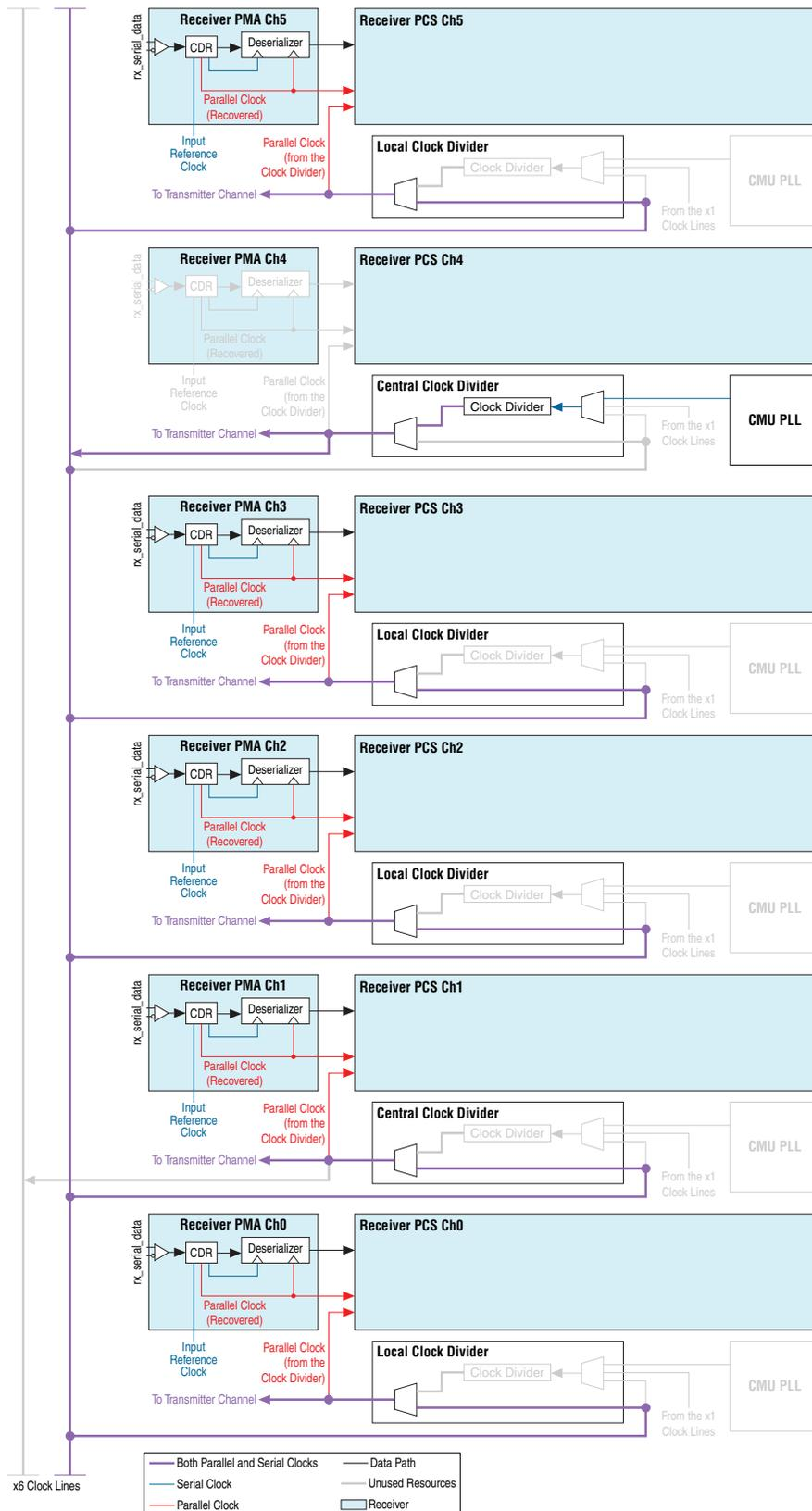
Figure 2-19. Six Channels Configured in Bonded Configuration Using Fractional PLL
