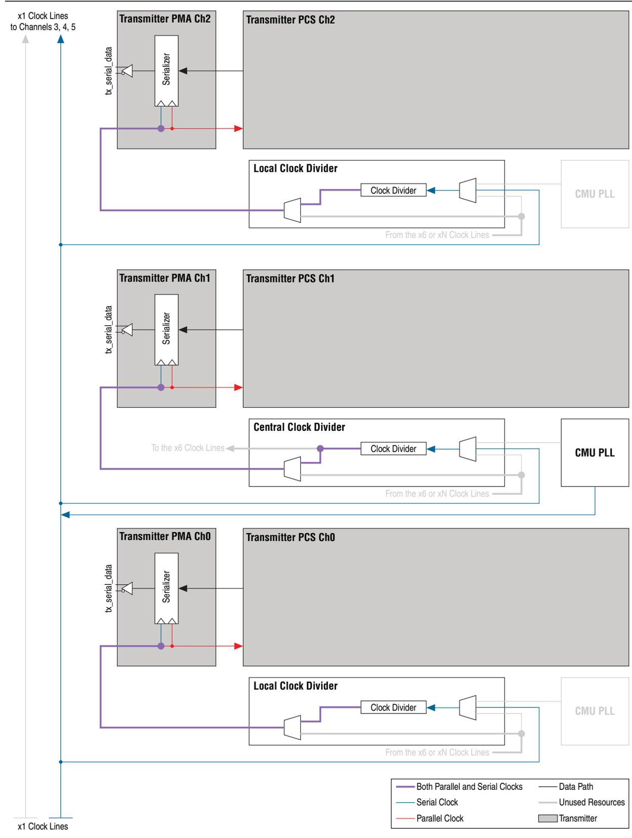
In non-bonded configurations for 10-Gbps transceivers, the local clock divider of the individual channel generates the parallel clock for the transmitter. In [Figure 2-12 on page 2-14](#), four 10-Gbps transmit channels function independently and are driven by their respective CMU PLL from the inactive 6-Gbps channels in the same triplet. The clock divider of each 10-Gbps channel generates its own parallel clock by dividing the serial clock coming from the CMU PLL of the same triplet.
