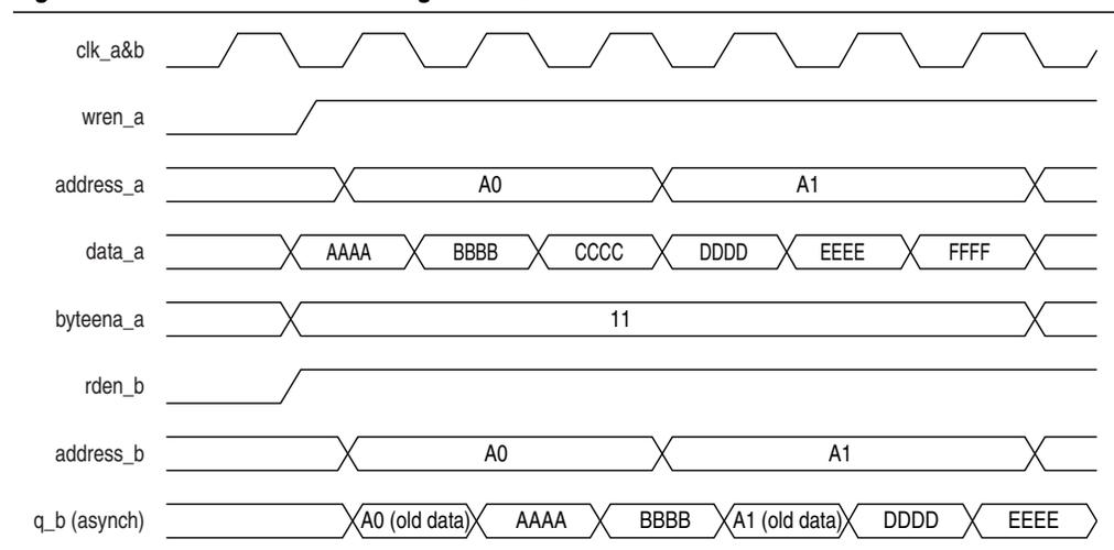
Figure 2-6 shows a sample functional waveform of mixed-port read-during-write behavior for the “don’t care” or “constrained don’t care” mode.
