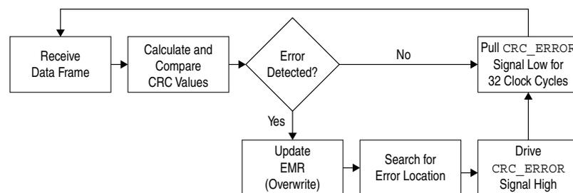
The error detection circuitry continues to calculate the 32-bit error detection CRC value and 32-bit signatures for the next frame of data regardless of whether an error has occurred in the current frame or not. You must monitor the CRC\_ERROR signal and take appropriate actions if a CRC error occurs.
