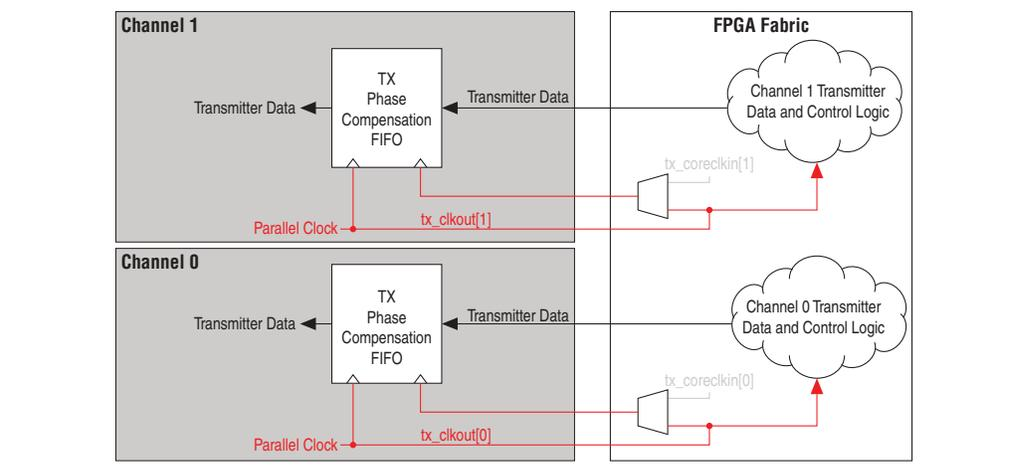
Figure 2-23 shows the transmitter datapath interface of two 10-Gbps transceiver non-bonded channels clocked by their respective transmitter PMA clocks, which are forwarded to the FPGA fabric.
