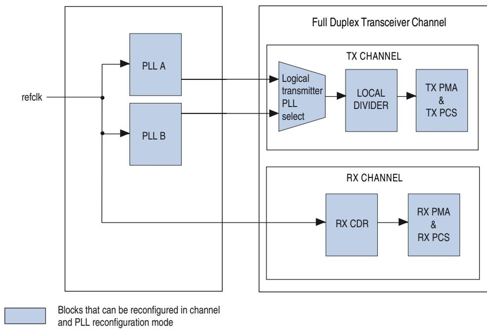
For more information about the transceiver channel and PLL reconfiguration, refer to the “Channel and PLL Reconfiguration” section in the *Transceiver Reconfiguration Controller* chapter of the *Altera Transceiver PHY IP Core User Guide*.
