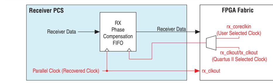
All configurations that use the PCS channel must have a 0 ppm difference between the receiver datapath interface clock and the read side clock of the RX phase compensation FIFO.
