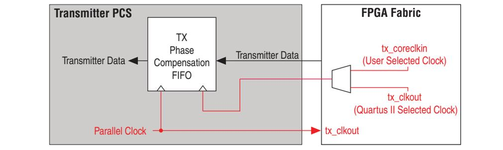
All configurations that use the PCS channel must have a 0 parts per million (ppm) difference between write and read clocks of the transmitter phase compensation FIFO.
