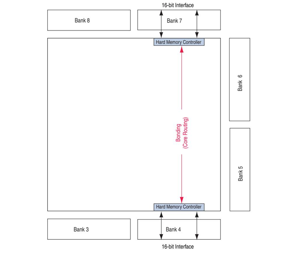
Figure 7-19 shows the bonding of opposite and same side hard memory controllers through the core fabric.
