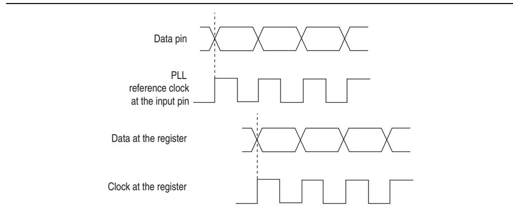
Source synchronous mode compensates for the delay of the clock network used and any difference in the delay between the following two paths:
