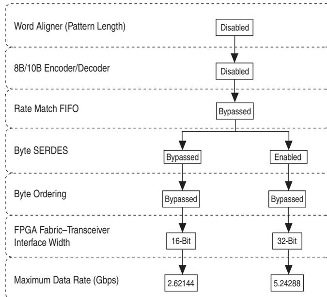
**Figure 5-18. Configuration Options for Low Latency Custom Double-Width Mode (20-bit PMA-PCS Interface Width)**
