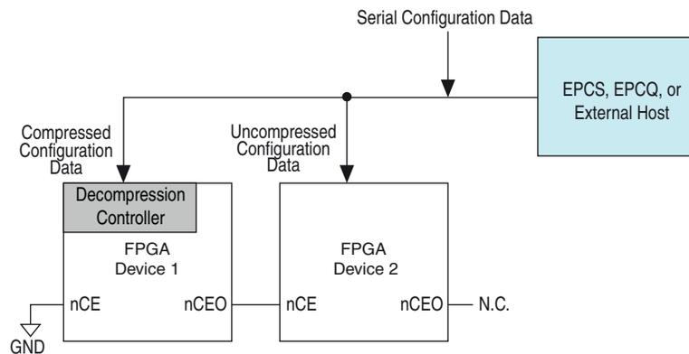
For the FPP configuration scheme, a combination of compressed and uncompressed configuration in the same multi-device configuration chain is not allowed because of the difference on the DCLK-to-DATA [ ] ratio.
