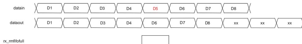
Figure 5-9 shows the rate match FIFO empty condition in custom single-width mode. The rate match FIFO becomes empty after reading out data byte D3.
