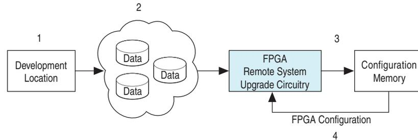
You can design your system to manage remote upgrades of the application configuration images in the configuration device. The following list is the sequence of the remote system upgrade:
