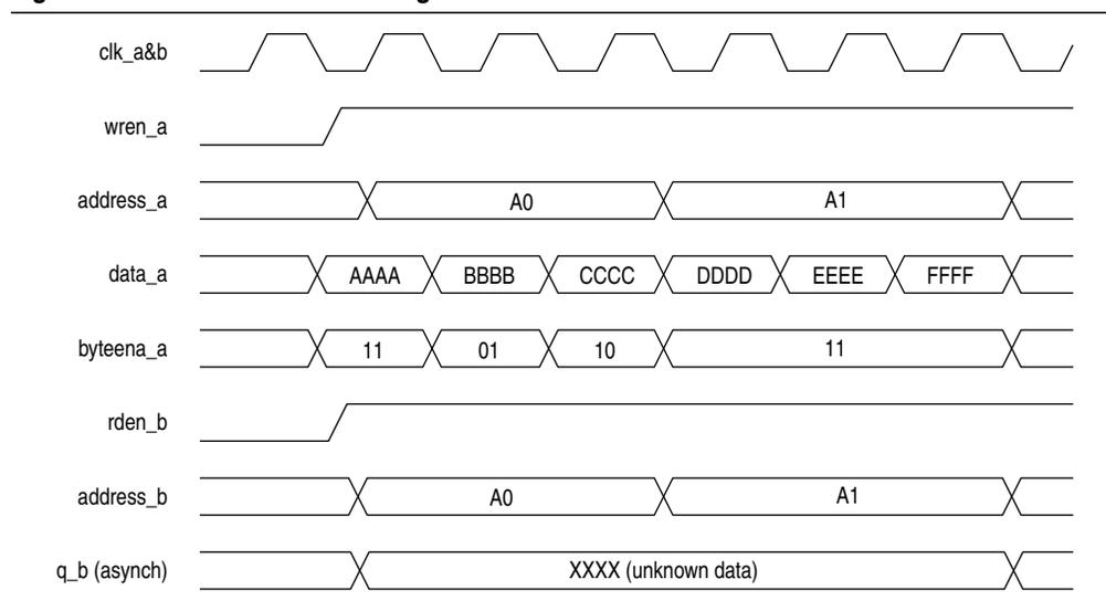
In the dual-port RAM mode, the mixed-port read-during-write operation is supported if the input registers have the same clock. The output value during the operation is “unknown.”
