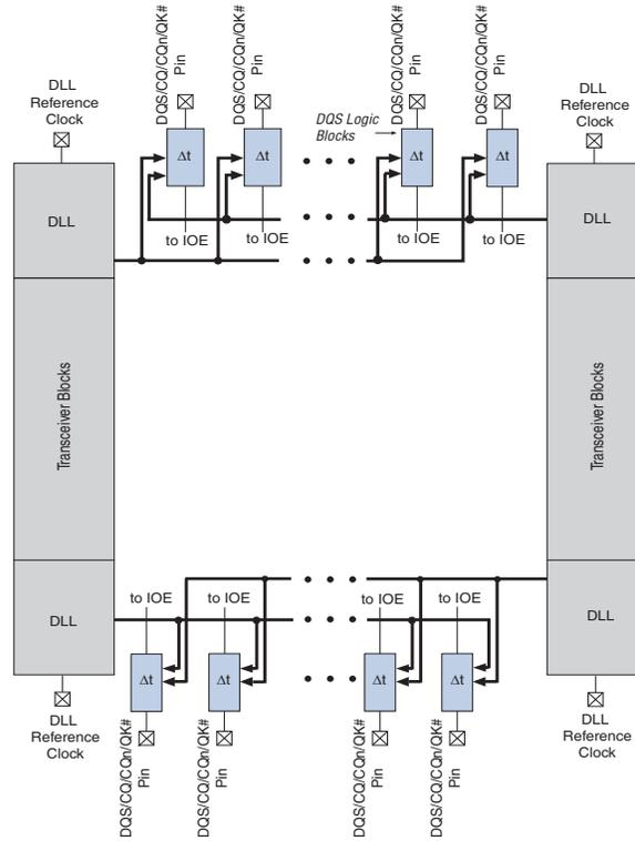
**Figure 7-4. DQS/CQ/CQn/QK# Pins and DLLs in Arria V SX B3 and B5 Devices, and Arria V ST D3 and D5 Devices—Preliminary**
