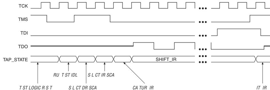
From the RESET state, TMS is clocked with the pattern 01100 to advance the TAP controller to the SHIFT\_IR state. The TDO pin is tri-stated in all states except in the SHIFT\_IR and SHIFT\_DR states. The TDO pin is activated at the first falling edge of TCK after entering SHIFT\_IR or SHIFT\_DR state and is tri-stated at the first falling edge of TCK after leaving SHIFT\_IR or SHIFT\_DR state.
