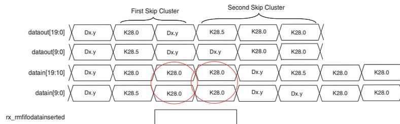
Figure 5-12 shows the rate match FIFO full condition in custom double-width mode. The rate match FIFO becomes full after receiving the 20-bit word D5D6.
