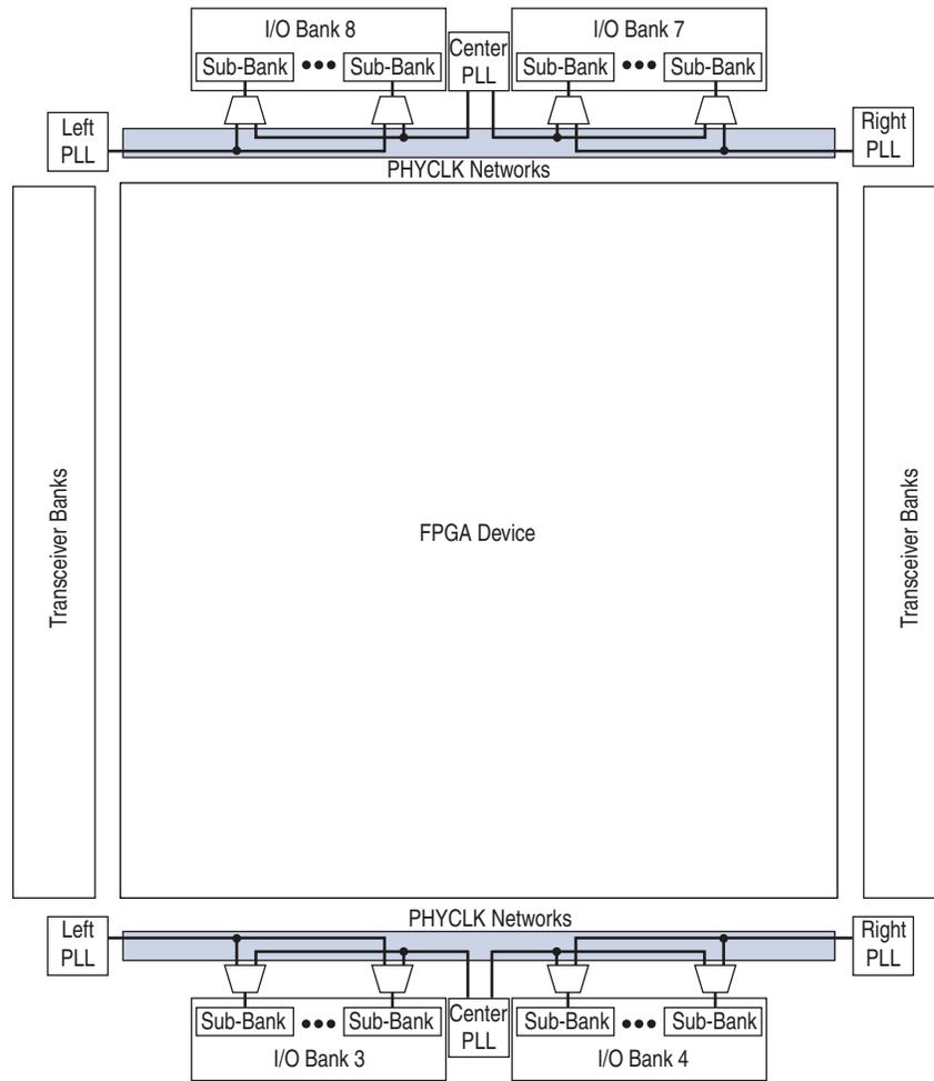
Figure 7-8. PHYCLK Networks in Arria V SX B3 and B5 Devices, and Arria V ST D3 and D5 Devices
