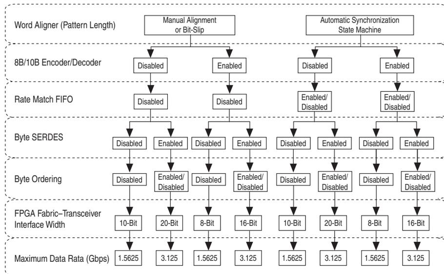
**Figure 5-4. Configuration Options for Custom Double-Width Mode (16-bit PMA-PCS Interface Width)**
