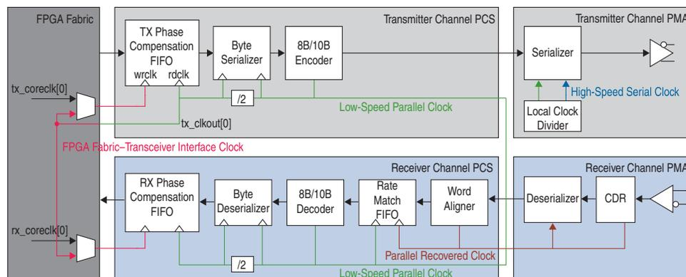
Arria V transceivers support SRIO physical layer specifications, versions 1.3 and 2.1, from 1.25 Gbps to 6.25 Gbps. The transceivers are compliant with the x2 and x4 channel bonding, deskew state machine, and rate match FIFO.
