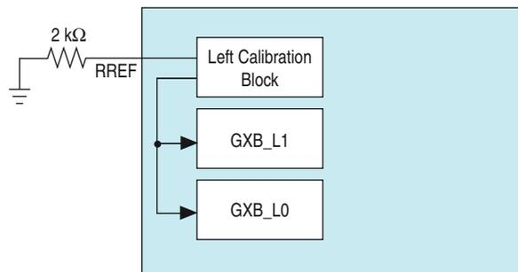
**Figure 1-16. Calibration Block Location and Connections in Arria V Devices with Transceivers on Both Sides of the Device**
