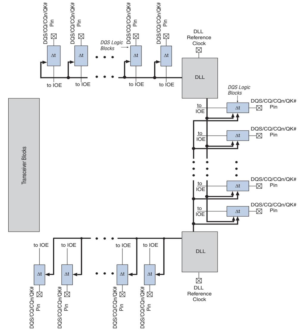
**Figure 7-3. DQS/CQ/CQn/QK# Pins and DLLs in Arria V GX B1, B3, A5, A7, B5, and B7 devices, and Arria V GT D3 and D7 Devices**
