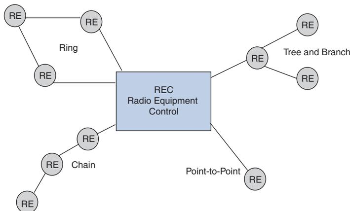
If the destination for the high-speed serial data that leaves the REC is the first RE, it is a single-hop connection. If the serial data from the REC must traverse through multiple REs before reaching the destination RE, it is a multi-hop connection.
