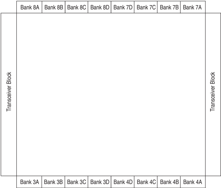
Figure 5-2. I/O Banks for Arria V GX A5, A7, B1, B3, B5, and B7 Devices, and Arria V GT C7, D3, and D7 Devices (1) —Preliminary
