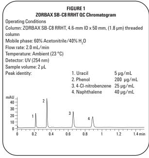
The uniform, spherical, ZORBAX SB-C8 particles have a controlled pore size of 80Å. Columns are loaded to a uniform bed density using a proprietary, high-pressure, slurry-loading technique to give optimum column efficiency.
