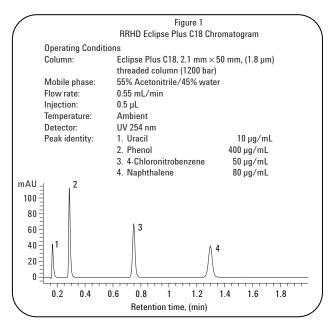
The efficiency reported on the Column Performance Report may be higher than the efficiency found in your laboratory. The QC test system may vary from the LC used in your lab and has been modified from a standard system to minimize the system volume. This allows a better evaluation of the packed column and assures a more consistent product for the chromatographer.
